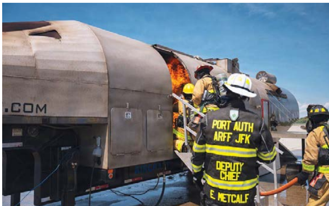
Firefighters enter a mobile aircraft fire trainer for live fire training at Stewart Air National Guard Base, N.Y., May 5. The fire department held the live fire training with the help of the Port Authority fire department to strengthen fire response readiness and tactics.
