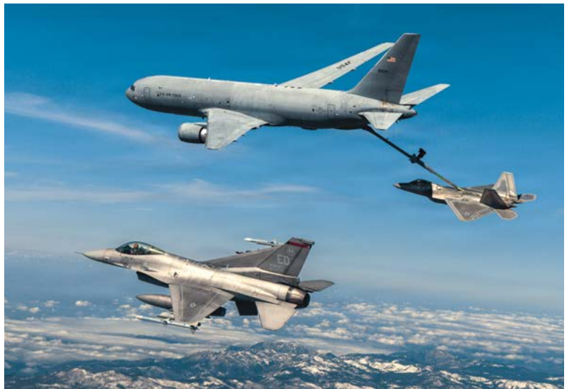
A KC-46 Pegasus refuels an F-22 Raptor over the Mojave Desert, while an F-16 awaits its turn in March.
