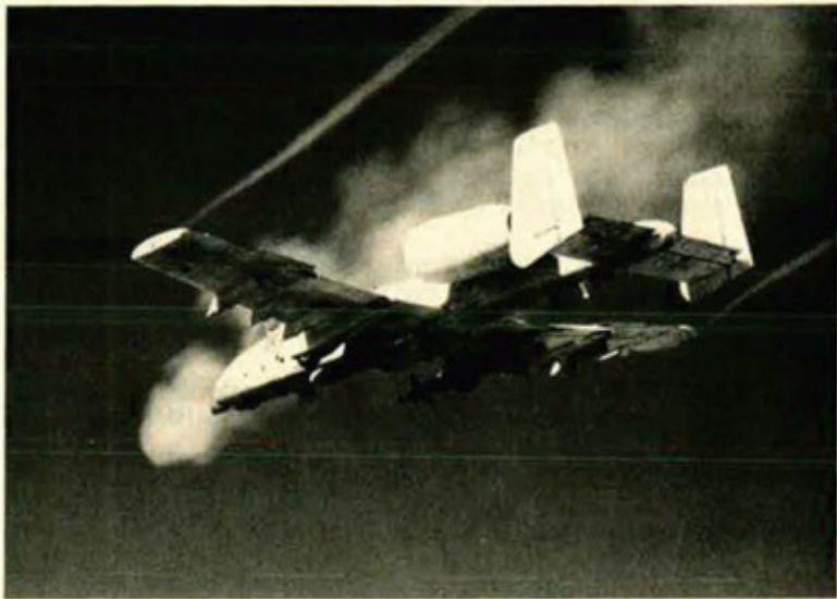
At the Air Force Flight Test Center, Edwards AFB, Calif., an A-10's GAU-8 30-mm cannon is put through its paces firing production ammunition. The GAU-8, largest gun ever mounted in a US fighter or attack aircraft, will make the A-10 a lethal tank killer.
