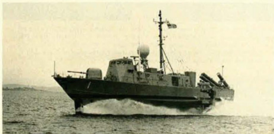
Above, finishing touches are put on scale test model of the Space Shuttle orbiter by employees at Rockwell International Corp.'s Los Angeles Aircraft Div. Built for Rockwell's Space Div., the model will be used for wind-tunnel tests at NASA's Ames Research Center, Calif. Below, US Navy's new missile ship Pegasus is the first of a line of Patrol Hydrofoil Missile ships (PHMs). Built by Boeing Aerospace Co., she'll undergo evaluation on the Pacific Missile Range. For an appraisal of the Navy's current and future combat strength, see p. 34 of this issue.
