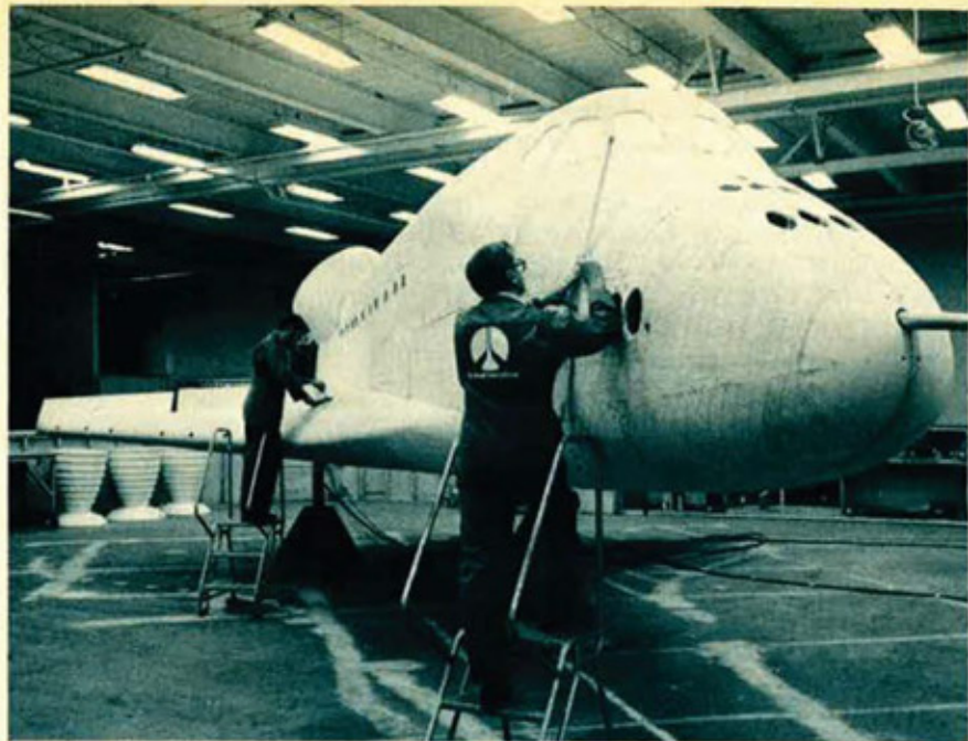
Above, finishing touches are put on scale test model of the Space Shuttle orbiter by employees at Rockwell International Corp.'s Los Angeles Aircraft Div. Built for Rockwell's Space Div., the model will be used for wind-tunnel tests at NASA's Ames Research Center, Calif. Below, US Navy's new missile ship Pegasus is the first of a line of Patrol Hydrofoil Missile ships (PHMs). Built by Boeing Aerospace Co., she'll undergo evaluation on the Pacific Missile Range. For an appraisal of the Navy's current and future combat strength, see p. 34 of this issue.
