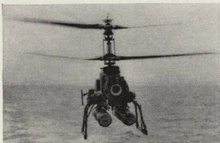
DASH , torpedo-carrying anti-submarine helicopter, operational with U.S. Navy, is powered by Boeing T50 gas turbine engine.
