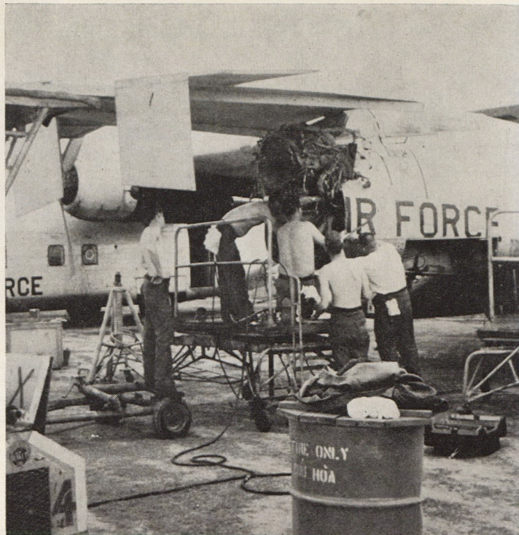
A damaged nose section of an F-100 gets rapid on-site repair job from Air Force Logistics Rapid Area Maintenance (RAM) team in Vietnam. AFLC field teams are composed mostly of civilians. They expedite the removal, recovery, and repair of crash- and battle-damaged aircraft.
