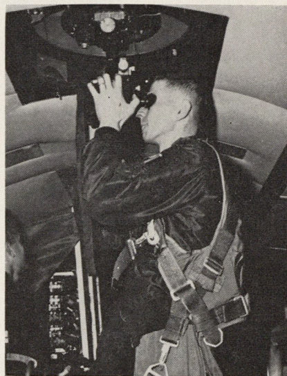
USAF trains its navigators in a "Flying Classroom." It is a transport, fitted with periscope sextants in ceiling. Here a student takes fix on stars as exercise.
