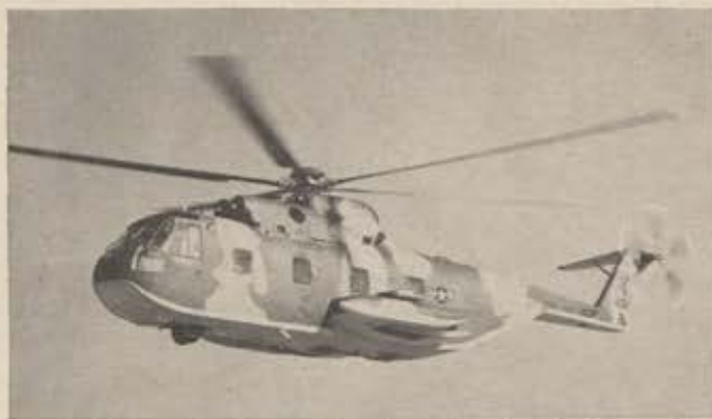
Destined for Air Rescue Service units in Southeast Asia, this Sikorsky HH-3C helicopter has just been delivered to USAF. More powerful than standard CH-3C, which has been in USAF service since 1963, HH-3C is armor plated and is equipped with additional communications and rescue gear.
