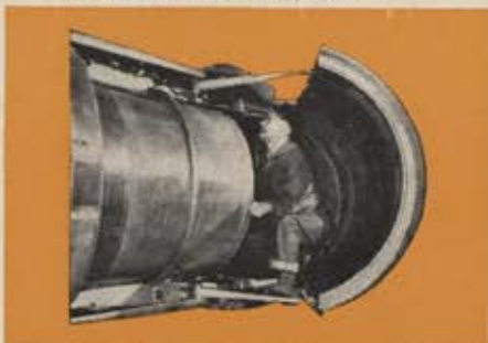
Rohr-designed and Rohr-built Thrust Reverser for the Lockheed C-141 — in service since December, 1963.
