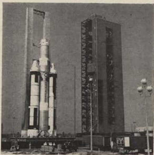
USAF's Titan III-C booster, which has already shown its multimillion-pound thrust, is also progressing well. Above, at Cape Kennedy's Complex 41 a fully assembled launch-ready bird is checked out by Martin Co.
