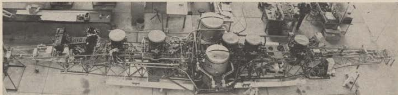
The flying testbed of the VAK 191B V/STOL fighter, shown above, is in its last stages of construction and may have already flown when this article goes to press. It is built around three engines. There are two Rolls-Royce Rb. 162 lift engines and one Rb. 193 vectored-thrust turbofan, all of which will be installed in the fuselage. No existing V/STOL aircraft has this mixed-propulsion concept, which sacrifices payload for operational safety.
