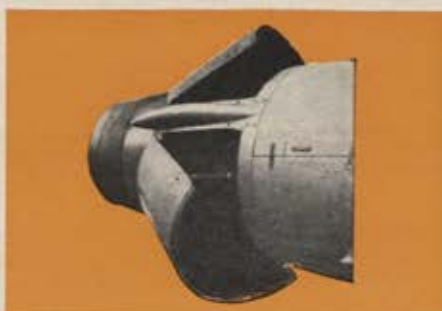
Rohr-built Thrust Reverser for the Boeing 727 — in service since February, 1963.
