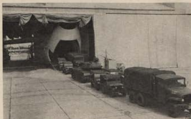
Cargo capacity of C-5A is illustrated in this demonstration conducted with Lockheed's mockup. More than ninety percent of the Army's equipment can be accommodated, including the mobile sixty-ton-plus "scissors" bridge for rapid tank assault across ravines, tanks, heavy helicopters, etc.
