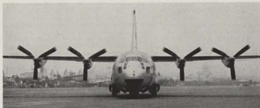
The smiling mouth on this Lockheed C-130 is a plastic radome. The happy-appearing turbo-prop transport is now undergoing flight testing for the AF.
