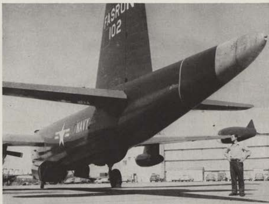
The long, pointed tail on this Navy Lockheed P2V contains special apparatus for spotting submerged submarines. It registers magnetic field disturbances.
