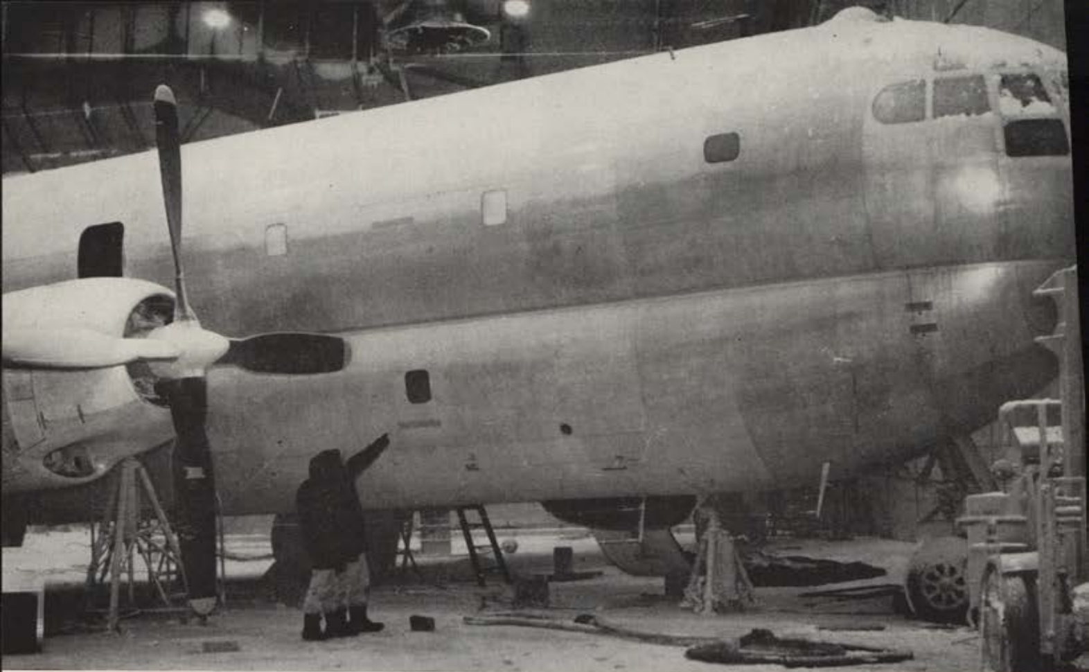
Air Force equipment can be tested at sixty-five degrees below zero in the climatic hanger at Eglin AFB, Florida.
