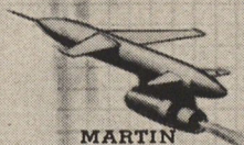
MARTIN KDM-1 ... U.S. Navy target drone... ramjet-powered, radar tracked, radiocontrolled.
