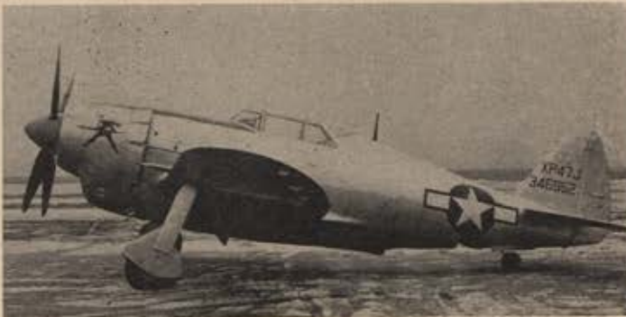
The J was powered by fan-cooled Wasp R-2800 with CH-5 supercharger.
