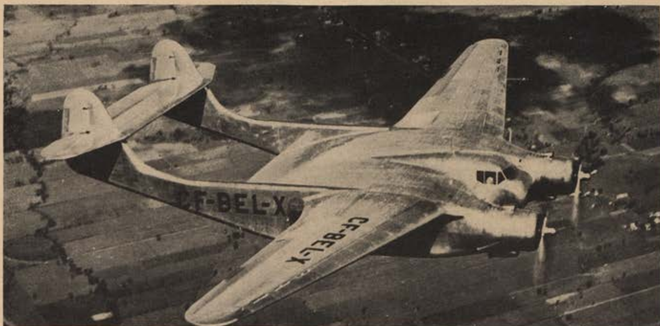
Flight view of the Burnelli CBY. This version, built in Canada, is rigged to carry cargo and passengers for back-country type operation.
