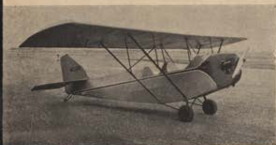
Minimum outlay and operating expense is typified by the Ross Sport. This craft has the simplest possible wing and fuselage structure, a 65-hp engine and a rigid landing gear, which uses full-air wheels for shock absorption. It is considered by some to be the last of the true light airplanes.
