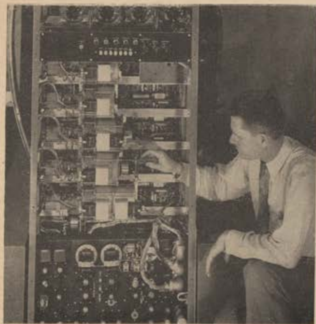
Dr. Dehmel, inventor of the Curtiss-Wright electronic trainer (below), checks the recording stylus on the special setup for P-38s. The device reproduces the characteristics of the airplane by means of electronic circuits controlled by potentiometers. The arrangement of the electronically controlled mechanism which computes the instrument indications for the new trainer is shown at left. Picture shows the technician pointing out one of the automatic servo-mechanisms.
