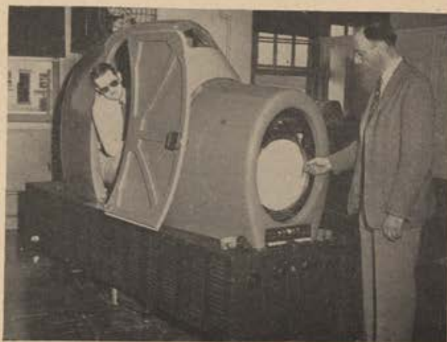
Dr. Dehmel, inventor of the Curtiss-Wright electronic trainer (below), checks the recording stylus on the special setup for P-38s. The device reproduces the characteristics of the airplane by means of electronic circuits controlled by potentiometers. The arrangement of the electronically controlled mechanism which computes the instrument indications for the new trainer is shown at left. Picture shows the technician pointing out one of the automatic servo-mechanisms.
