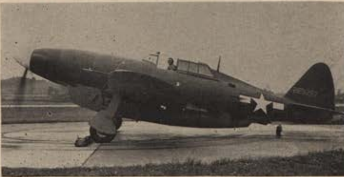
XP-47H, test bed for Chrysler's 2500-hp experimental engine.
