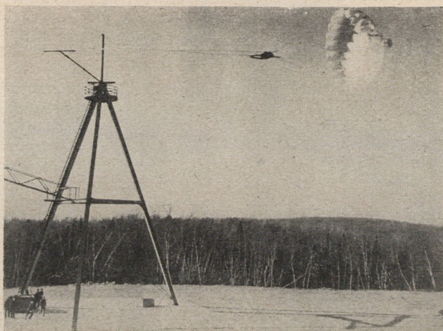
Mounted atop 120-foot high pylon, a parachute with a man-size dummy is whirled in tests to determine high-speed bailout data.
