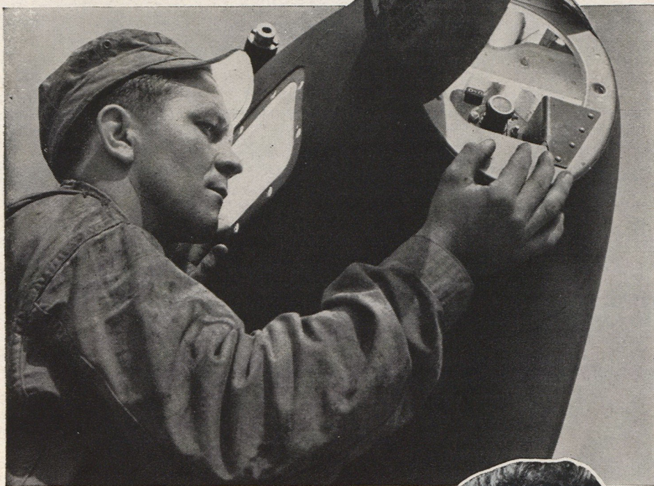
This small movie camera in the nose of a P-38 is used as an aid in improving firing accuracy. Visible in the photo above are three .50 caliber machine guns and one 20 mm cannon.
