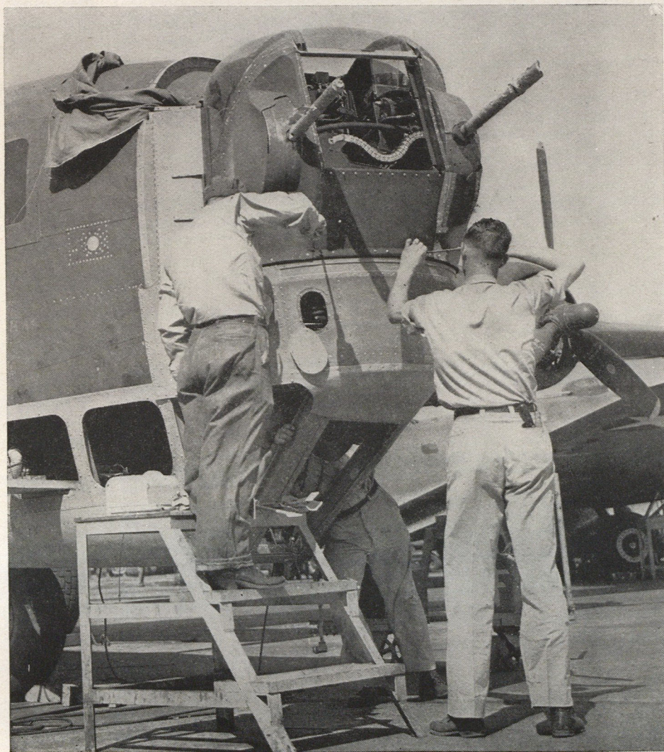
Oklahoma City Air Depot workers fasten the final bolts and screws in mounting a new stinger in the nose of a B-24. The glass front pieces are installed after the turret is tightened in place.
