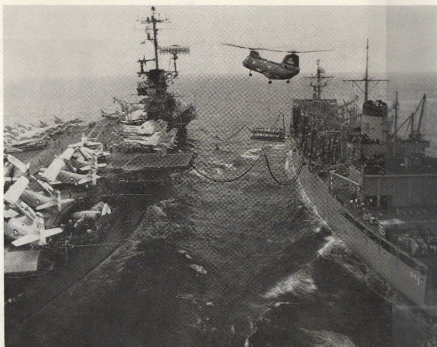
For the past two years the U.S. Navy has employed UH-6 Sea Knight helicopters to cut sharply the time needed for transfer of supplies. One is shown here carrying fuel tanks from the USS SACRAMENTO, at right, to the USS HANCOCK off Vietnam.
