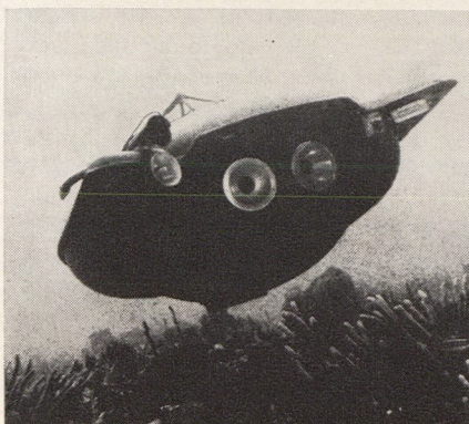
Westinghouse Electric Corporation has designed a research submersible which it hopes will be able to dive to 20,000 feet (6,096 m). The "Deepstar," above, has been successfully tested, diving to a depth of 4,000 feet (1,200 m), exploring the ocean floor for 90 minutes, and demonstrating its maneuverability by picking up samples of animal life.
