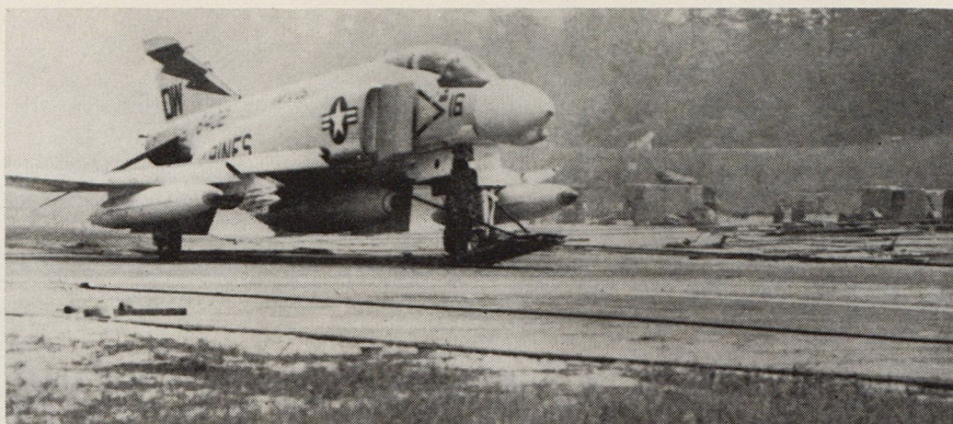
A Marine Corps F-4 begins its takeoff run on the CEI-3 aircraft catapult, part of the SATS (Short Airfields for Tactical Support) program now in service at the Chu Lai Air Base in Vietnam. The system was developed by All American Engineering Company. For more on the SATS system, see the article beginning on page 34 of this issue.
