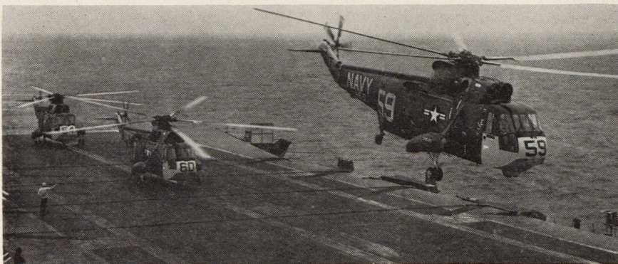
Though normally employed for antisubmarine patrol, Sikorsky SH-3A Sea King helicopters, with ASW gear removed, are now operating from U.S. Navy carriers in the Gulf of Tonkin to assist in rescuing aircrews who bail out of disabled aircraft.
