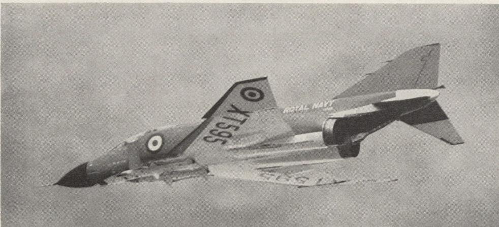
The British are scheduled to receive 290 Phantom IIs for the Royal Navy and Royal Air Force. They will be powered by Rolls-Royce Spey turbofan engines and will have substantially better range than USN and USAF versions.
