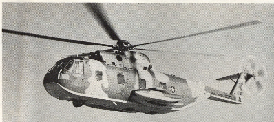
Capable of in-flight refueling for long-range rescue operations is the Air Force's HH-3E "Jolly Green Giant." It is similar to the Sikorsky CH-3C transport helicopter but employs a more powerful engine and special communications and rescue equipment.
