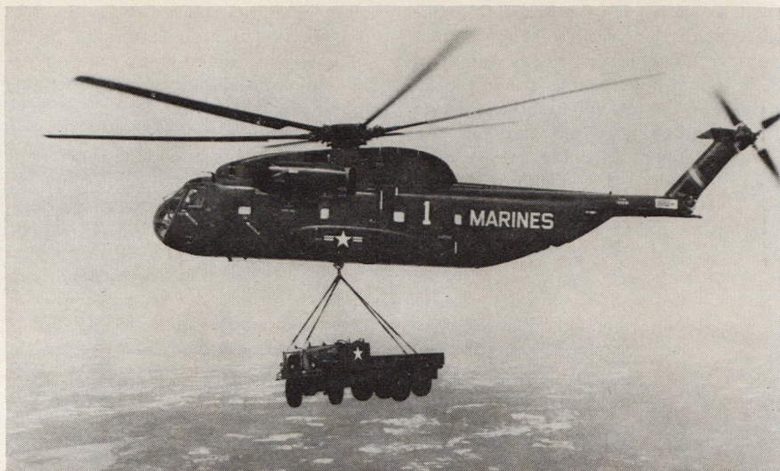
Biggest, heaviest, and fastest U.S. helicopter now in production is the Sikorsky CH-53A Stallion assault transport, which the Marine Corps expects to introduce into Vietnam operations late this year to supplement and later replace its CH-34 Choctaws. Meanwhile, the U.S. Air Force has ordered an air rescue version of the Stallion, designated HH-53B, with longer range and higher speed than its HH-3E Jolly Green Giant.
