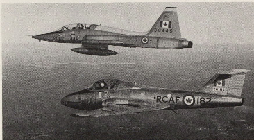
First photo of these Canadair-built jet planes in formation flight shows Northrop CF-5 tactical fighter, above, with CL-41 Tutor trainer. Montreal-based Canadair Ltd. has entered into production of 125 CF-5s for Royal Canadian Air Force. CL-41, featuring side-by-side seating, is the first trainer RCAF cadets fly. The Royal Malaysian Air Force has ordered 20 of a tactical fighter/trainer version, designated the CL-41G.
