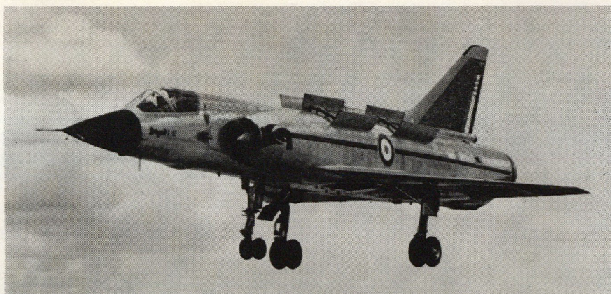
First VTOL aircraft to reach speed above Mach 2 in level flight is Dassault Mirage IIIV. Flown by Dassault test pilot Jean-Marie Saget, the second of four prototypes in development program was clocked at Mach 2.04 on its eleventh flight September 12. Saget reported a very smooth transition from vertical to horizontal mode and back.
