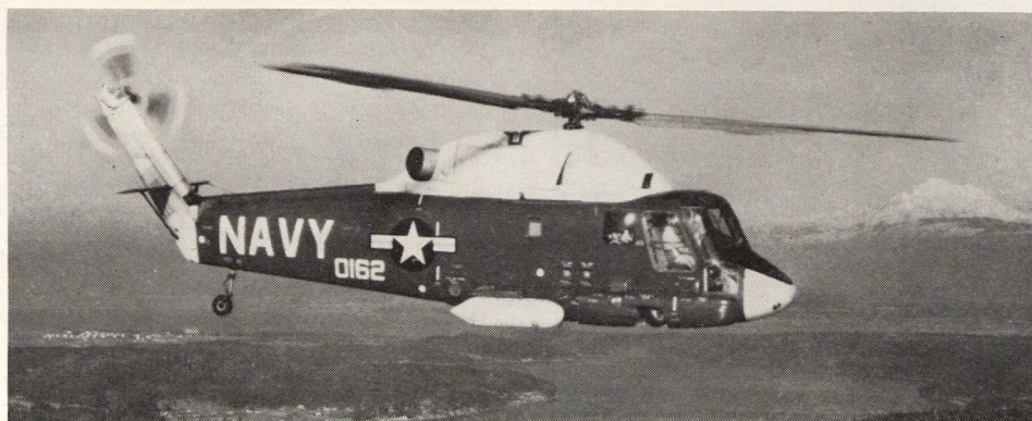
Closeup view of the Kaman UH-2B Seasprite, powered by a General Electric T58-8 engine with 1,250 shp. It has been fitted with 7.62-mm machine guns and armor plate for search and rescue operations off Vietnam.
