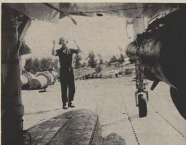
Heavily armed A-4 is directed out for takeoff at Chu Lai by Marine Pfc. Ray Markley. The aluminum matting forming the Chu Lai strip was laid on deep sand stabilized with asphalt. A portable arresting gear also has been installed.
