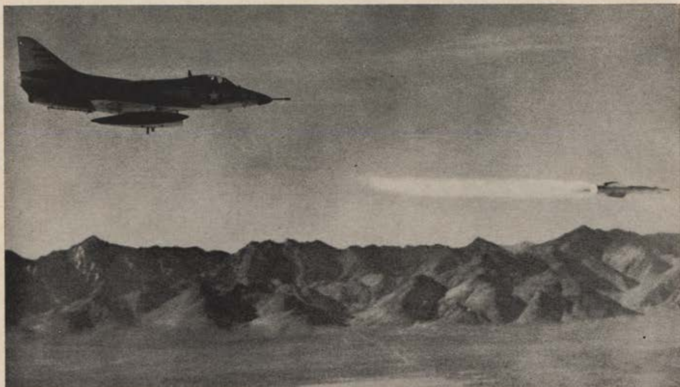
A wide variety of armament loads can be accommodated on the A-4. One of the most important weapons, the Martin Bullpup, is shown being launched above. The Bullpup has been used in action many times in Vietnam by A-4 pilots. They have used its radio guidance feature to destroy pinpoint targets such as radar antennas and concrete command posts.
