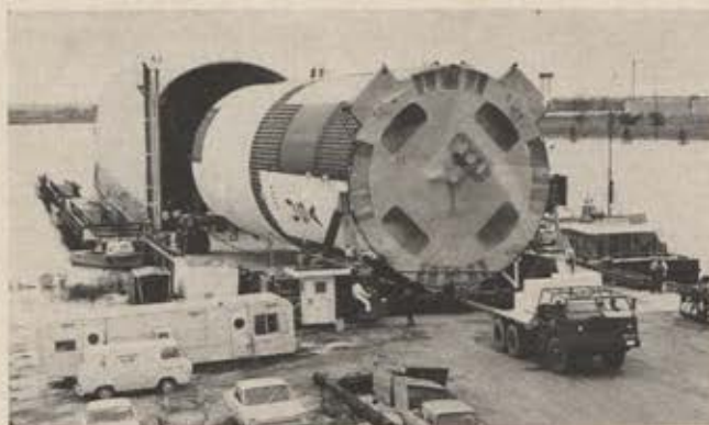
The first Boeing-built stage of the Saturn V booster is loaded aboard a barge at NASA's Michoud Assembly Facility near New Orleans, La., for shipment to the Marshall Space Flight Center at Huntsville, Ala., to undergo tests of its ability to withstand vibration, bending, and other stresses.
