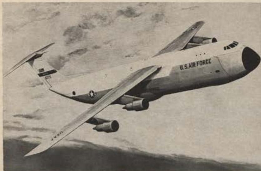
This is an artist's conception of how the USAF C-5A transport will look when it goes into service in 1969. Lockheed has been chosen to build the 700,000-pound aircraft and General Electric will furnish the four 40,000-pound thrust fanjet engines. C-5A's cubic capacity is one of its most important advantages. It is designed to carry bulk as well as tremendous weight.
