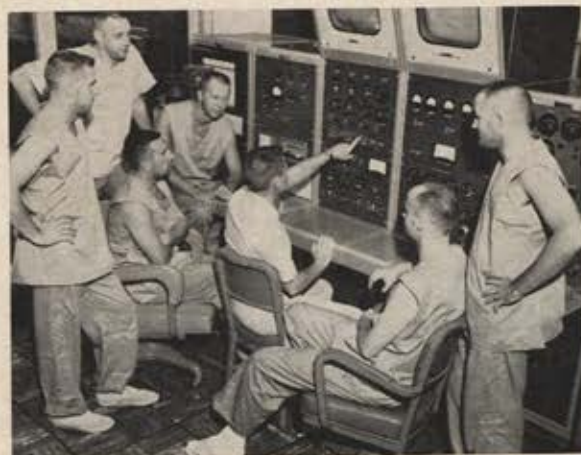
Volunteers at USAF's Aerospace Medical Center at Brooks AFB, Tex., are spending some sixty days in oxygen/helium atmosphere, testing the mixture for possible use in forthcoming MOL project. Above, team from which four-man crew was chosen is briefed. Simulated altitude, using seventy percent oxygen, thirty percent helium mix, will be 27,000 feet.
