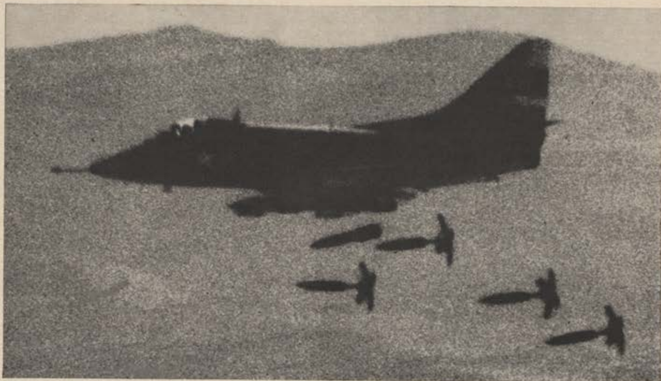
Snakeye bombs are among the new weapons being employed against the Viet Cong. The cross-shaped drag brake slows the bombs rapidly and allows the aircraft to pull away from them and escape blast damage during low-level attack. The A-4 also is equipped with two 20-mm. guns in the wings and others in pods to aid in low-level assault maneuvers.
