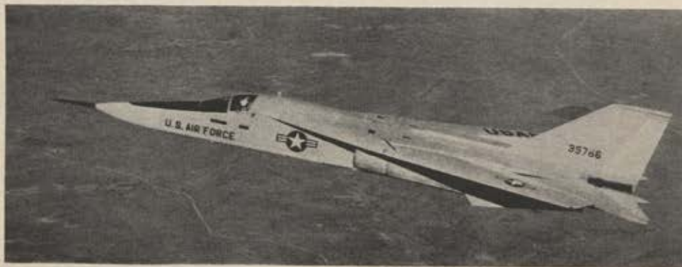
General Dynamics' variable-sweep wing F-111A was developed to meet requirement for a combat aircraft that can take off and land at relatively low speeds but can cruise at very high speeds and altitudes. Continuing evolution of the military airplane demands steady advances along the entire spectrum of aerospace technology.
