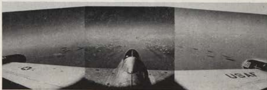
A rocket pattern blanketing an area as big as a football field is recorded by three cameras mounted in the tail of this Northrop F-89D Scorpion interceptor.
