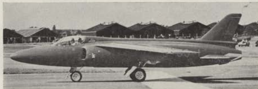
This tiny (6,000 lbs., 20-foot wingspan) Folland Midge jet fighter was shown at the recent SBAC show at Farnborough, England. Powered by an Armstrong-Siddeley Viper engine, it is capable of 600 mph. It is shown here at takeoff.
