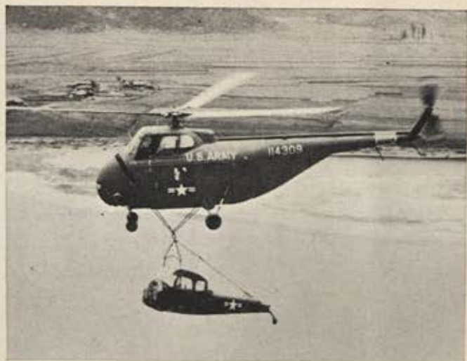
UNUSUAL CARGO —This crashed Army L-19 liaison plane was salvaged with ease in Korea by an Army Sikorsky H-19 helicopter. Two trips were needed to fly the damaged wings, engine and fuselage (above, in cargo sling) to a repair depot. Army Sikorsky helicopters are now solving hundreds of tough, unusual transportation problems.
