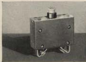
M.P. SERIES 80AE TRIP-FREE BREAKER Explosion-proof, arc resistant Melamine-Formaldehyde case. Yellow button, and fluorescent trip indication. Extended collar for edge lighted panels.
