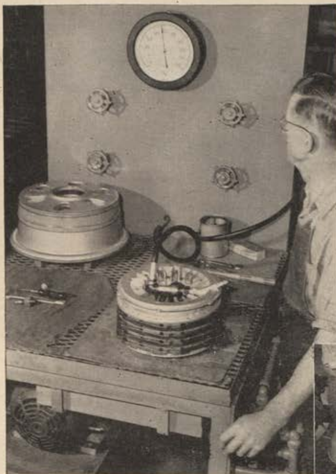
It measures up! Harvester simulates actual braking pressure under flight conditions to test every F-86 brake.
