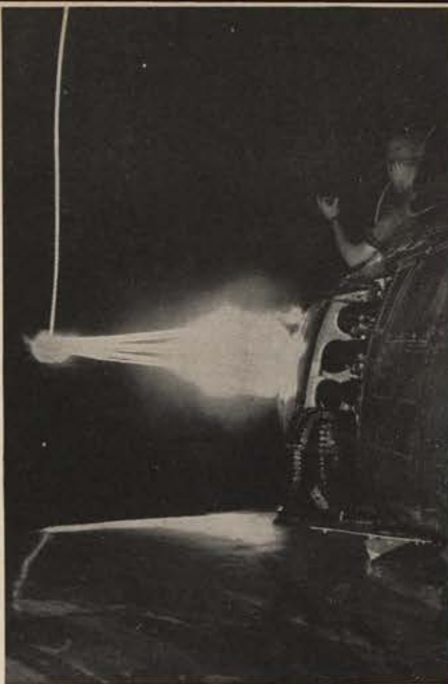
Six streams of .50 caliber slugs rip up the bulls-eye of a 51st F-1 target as an armament specialist synchronizes the gunsight of an F-86.
