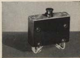
M.P. SERIES 60 NON-TRIP-FREE BREAKER Black Bakelite, flame retarding case. Black button. Radioactive luminescent, fluorescent trip indication. Approved for 115 volt, 400 cycles A. C. and 28-30 volt D. C. operation.
