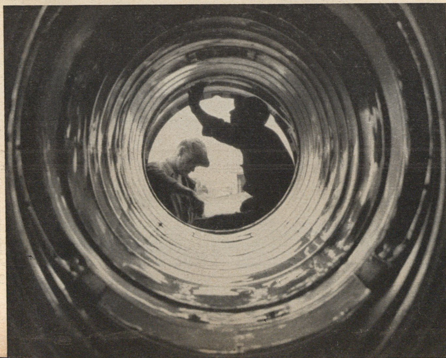
4. Below, an unusual study of Otis airmen inspecting cooling shroud which insulates the frame of their plane against intense heat of engine and tailpipe.
