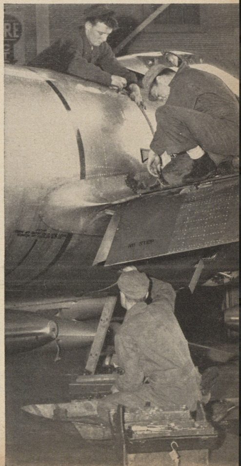
7. After satisfactory engine run-up, airmen replace tail section. Jet is now ready for its engineering test flight and return to the line.
