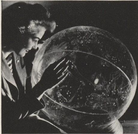
domes together, Colonel Davis cut in the latitude and longitude lines and drilled holes in the exact position of the stars in rough magnitudes. A fluorescent material was then sealed into the holes. In a dark room the stars glow and appear to twinkle. Allegorical figures were etched on the constellations for purposes of instruction.
