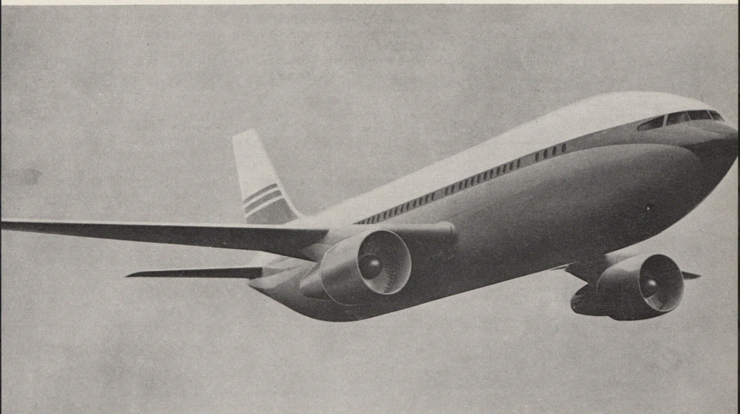
This is an artist's conception of the HBN-100 airbus proposal, developed by Hawker Siddeley, Breguet, and Nord-Aviation, for a two-engine airliner with a seating capacity of some 250 passengers, relatively short takeoff-and-landing characteristics, and some rather novel approaches to loading and unloading people and cargo. HBN-100 was chosen from a group of five varying airbus concepts.
