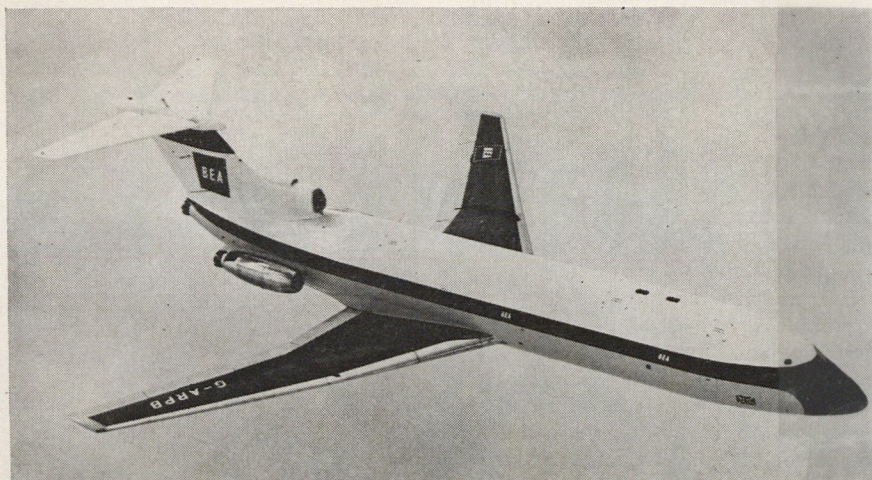
Hawker Siddeley's Trident, powered by three Rolls-Royce Spey engines, is flown by British European Airways, Pakistan International Airlines, Kuwait Airways, and Iraqi Airlines.
