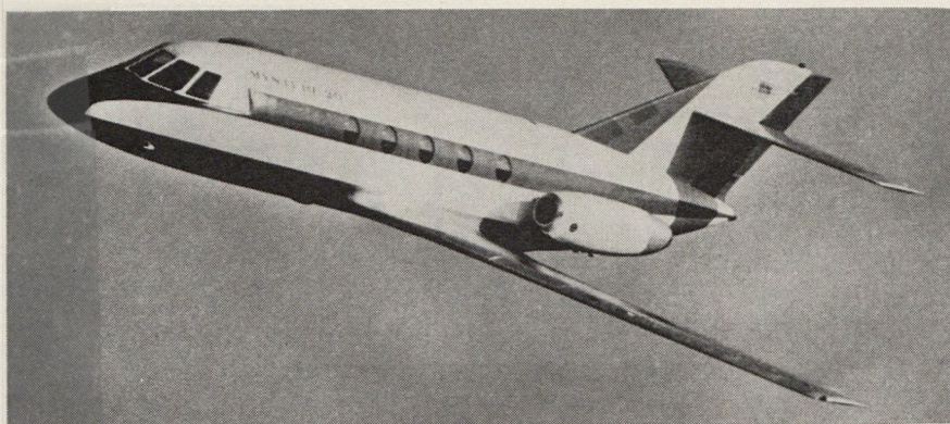
The Dassault-Sud Aviation Mystère 20, shown on its first flight, over Bordeaux, carries ten passengers, and can do 540 mph (870 km/hr). It has two Pratt & Whitney jet engines.
