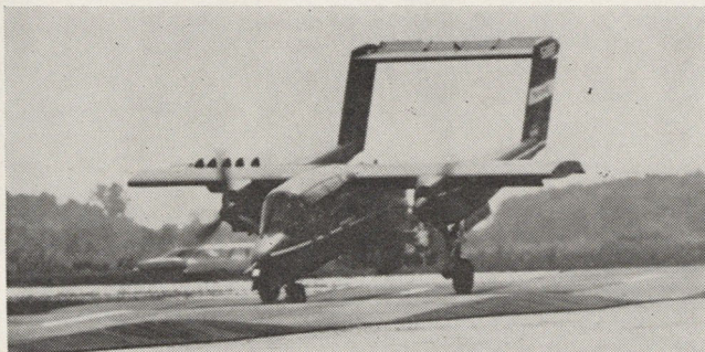
Pilots put North American OV-10A LARA through punishing tests on simulated rough airstrip at Naval Air Test Center, Patuxent, Maryland. At start of takeoff roll, plane's nose dips as nose gear encounters bump, but levels out on acceleration.
