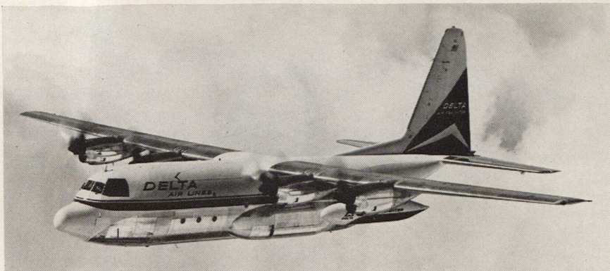
Lockheed-Georgia Company has launched a worldwide marketing campaign for its air freighters—the Lockheed-100, shown being delivered to Delta Airlines; the StarLifter; and the L-500. Four Allison turboprops of 4,050 shaft horsepower power the Hercules.
