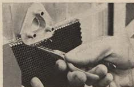
Honeycomb structure. Strips of metallic honeycomb must be cut to exact dimensions and bonded to surface of crew compartment. Over the honeycomb go sheets of aluminum alloy to form a tough, lightweight sandwich panel. Honeycomb technology, using aluminum, was first developed by North American for the F-86.
