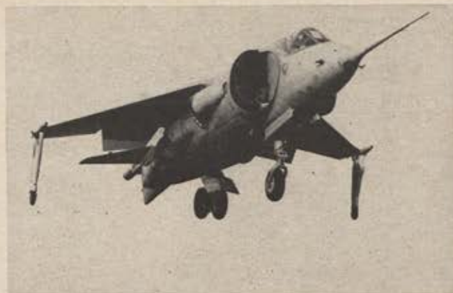
The Hawker Siddeley P.1127 V/STOL fighter, shown in vertical flight above, is probably the most advanced V/STOL aircraft in the world. Scheduled for military unveiling October 1, it has been flying for about three years and is close to its 2,000th successful takeoff and landing.
