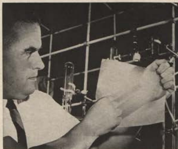
New fuel cell developed by General Electric features tough solid polymer, which increases life expectancy of system four to five times. Onboard power, as demonstrated by difficulties with Gemini-5 fuel cell system, is pressing technological requirement.
