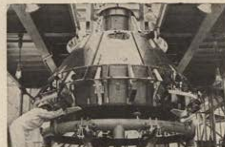
Final assembly. Mating of the two Apollo shells takes place in Building 290 at NAA/S&ID. This is the world's largest clean room—1,500,000 cubic feet of meticulously controlled air space. Here subsystems are installed. And here the completed command module is tested with service module and launch escape system.
