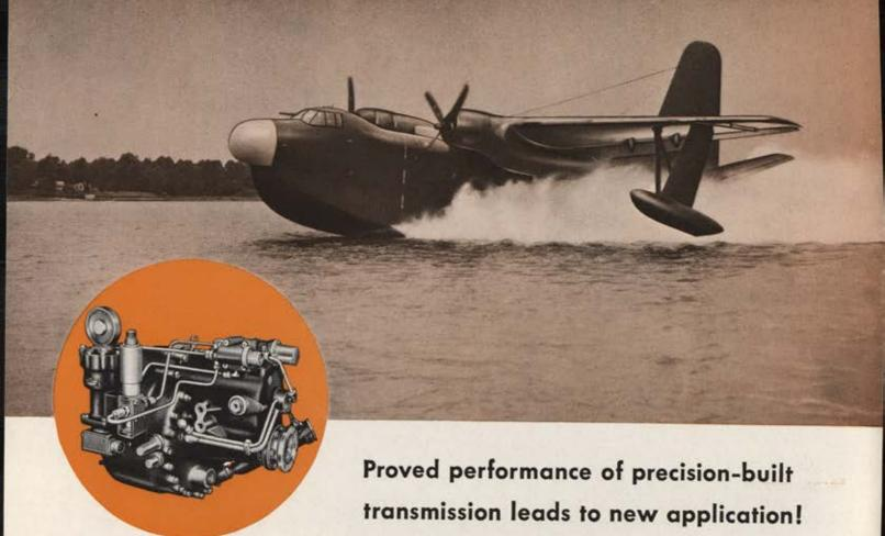
Due to the tremendous amount of electrical equipment required in this new, radar-loaded Martin P5M-1 Anti-Submarine Patrol Bomber, the availability of constant frequency AC current became a "must". This called for installation of Sundstrand Constant Speed Alternator Drives — a tried and proved method of providing weight-saving AC power in the air.
