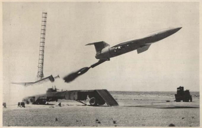
The B-61, launched from a tractor-drawn platform, gets an assist from a rocket dropped after flight speed is reached.
