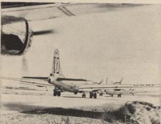
Taking off from Okinawa, the bombers head for high altitude. Heavy bomb loads and high altitude bombing are made possible by turbosuperchargers which give the B-29 extra power at altitude. Most modern piston-engined bombers, such as Boeing's B-50, Convair's B-36, and North American's AJ-1 use G-E turbos.
