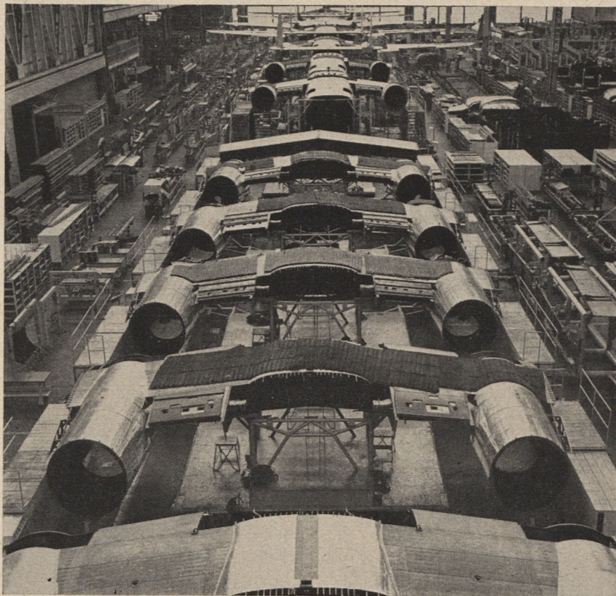
The joined halves of the center section move along the assembly line toward the finished airplanes. The two nacelles are ready to receive the engines and landing gear and in the next step, (bottom), is lowered into place on a fuselage. Soon the whole assembly will be on its wheels and on the way out.
