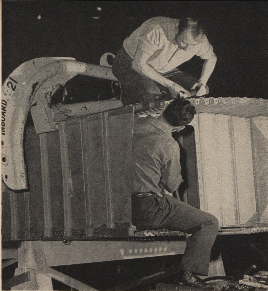
Workmen are shown above joining the two halves of the C-119 center section. Building the huge structure in two parts enables Fairchild to step up production on short notice. The sections are perfect units, already inspected.
