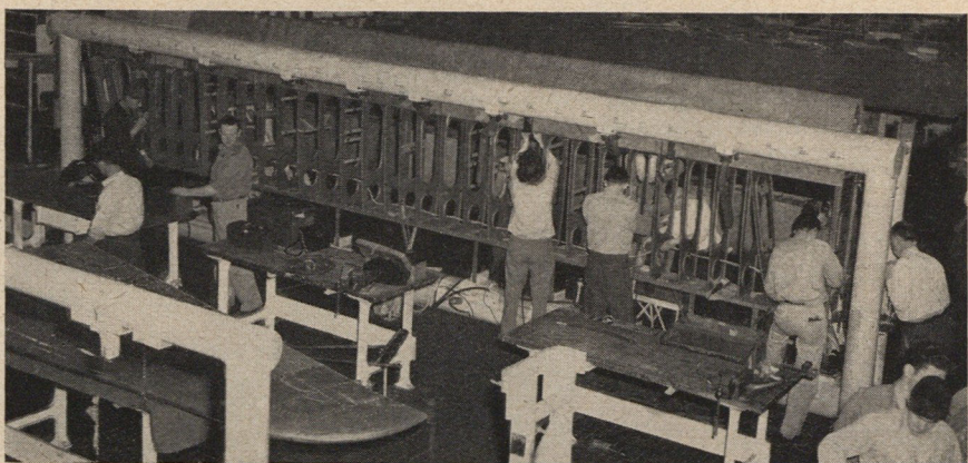
Skeleton of the horizontal stabilizer is assembled in a long jig (above). Some workers are inserting the ribs while others are installing electrical wiring before the aluminum skin is applied. Below a riveting machine goes to work on a section of the tail boom. In many instances large assemblies were broken into smaller units in order to utilize the mechanical riveter.
