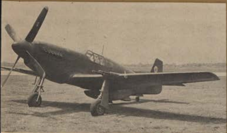
The P-51B, powered by a Packard-Merlin, carried 20mm cannon.
