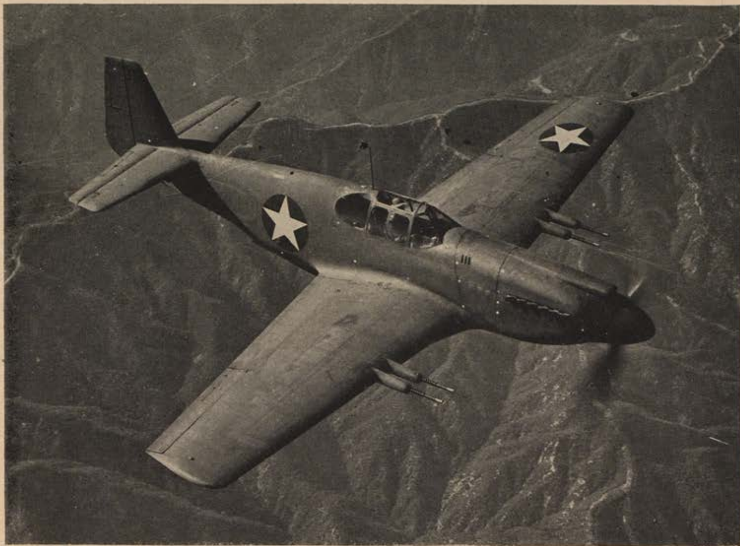
The P-51A was armed like the B, but was still powered by an Allison.
