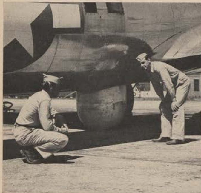
Radar men examine a "radome," a familiar appendage on the AAF's heavy bombers. The radome houses the "spinner" or parabolic antenna used to transmit radar waves and receive returning "echoes."
