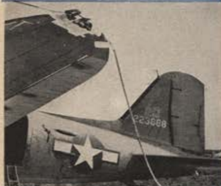
On the other plane, a hook and line arrangement is pinned to wingtip.
