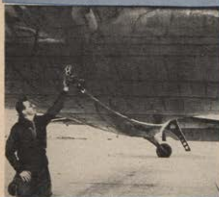
A glider tow mechanism and a line is fixed under plane to be towed.
