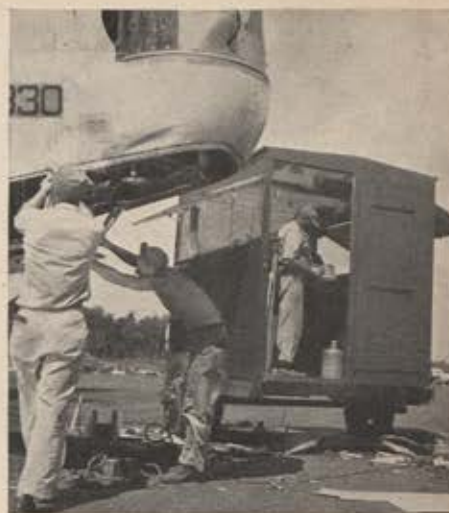
Each phase of maintenance is carried out by separate trailer in this mobile flight line. Above, 7th AF sheet metal men are at work.
