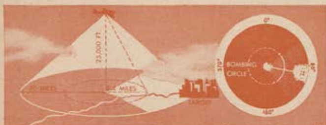
Irregular bright patch in PPI sketch at right shows how typical target might appear in radar scope set at 10-mile range. Straight white "Lubber Line" indicates true heading of plane toward target.
