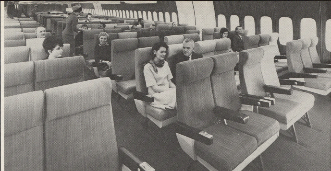
With a fuselage that's almost twice as wide as the largest contemporary jetliner, the 747 can accommodate up to 500 passengers easily and comfortably. Nine-or-ten-abreast seating, as shown here in Boeing's interior mockup of the 747, allows for two aisles and easy access to all seats. Operating economy of the 747 will be between 20 and 30 percent above that of the present generation of large jetliners. Runway requirements for Boeing's jumbojet airplane are said to be considerably better than those of the 707 or DC-8.
