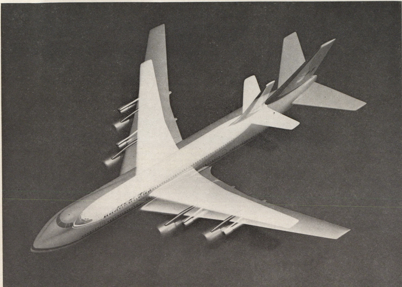
Scale model of the 747 dwarfs standard contemporary jetliner of the 707-320 class. Maximum gross weight is 680,000 pounds (308,440 kg) for the 747 and 328,000 pounds (148,780 kg) for the 707. The 747's top speed of 630 miles per hour (1,014 km/hr) exceeds that of the 707 by 30 mph (48 km/hr). Cruising almost one mile (1.6 km) above the operating ceiling of contemporary jetliners, the 747 can be expected to alleviate congestion in the high-traffic corridors in the U.S., in Europe, and over the Atlantic Ocean.
