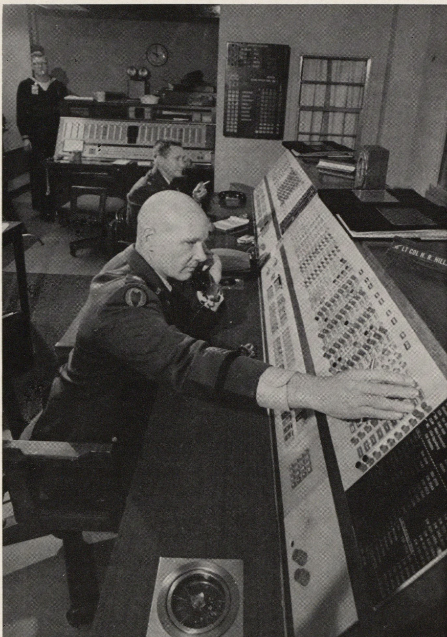
Inside the National Military Command Center in the basement of the Pentagon is the central control board for telephone communications. The room is packed full of radio and teletype machines in addition to the telephone system. One telephone is the "hot-line" link to Moscow. This is where command and control of U. S. Armed Forces starts.
