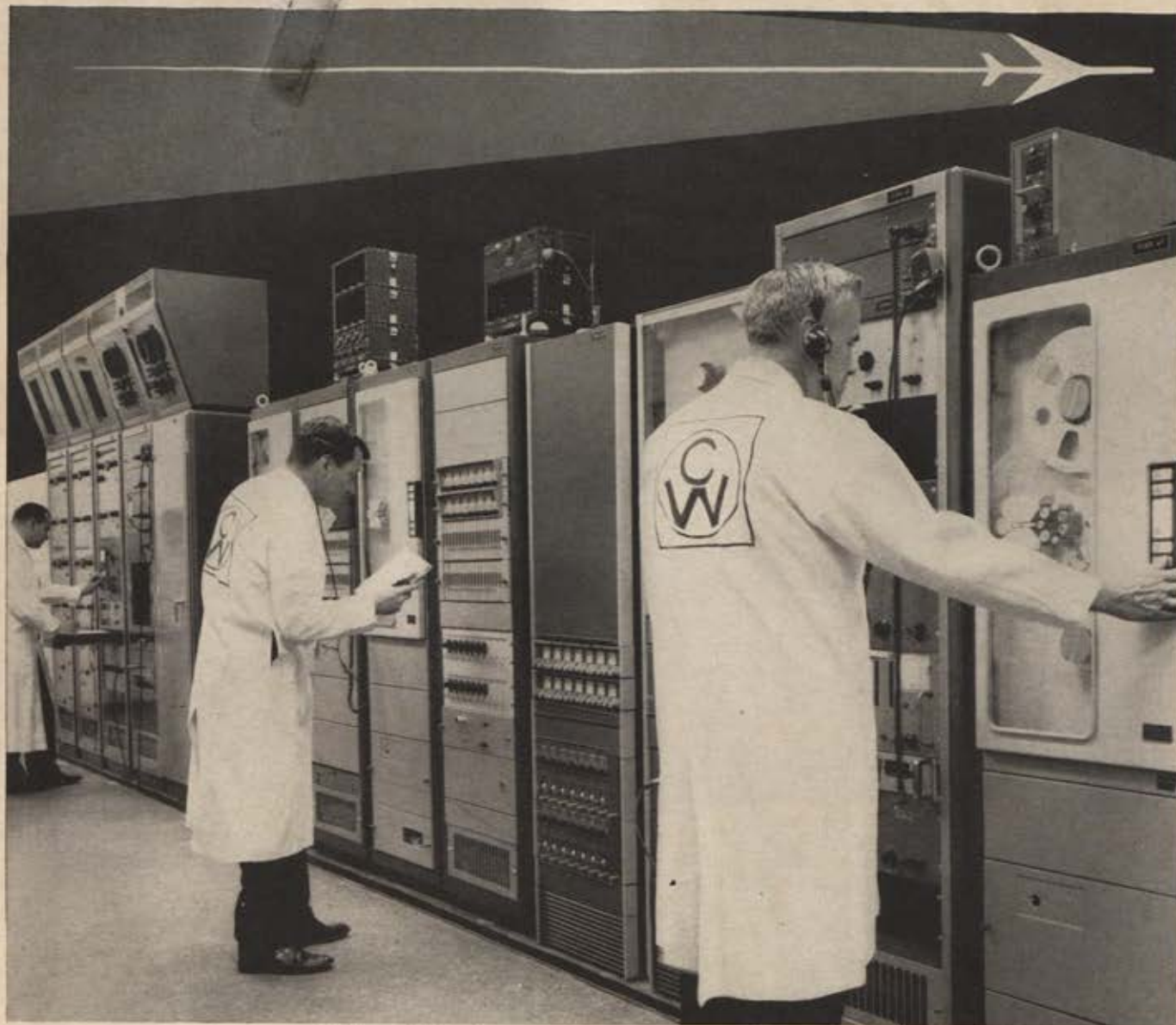
High-speed Automatic Data Recorders shown monitoring performance of U. S. Air Force development engine during test.
