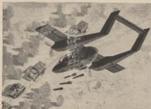
Carry 2,400 pounds of external stores—bombs, napalm, and four 7.62 mm machine guns with a total of 2,000 rounds.
