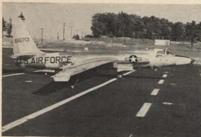
This Lockheed U-2 played an important part in OAR's Project Stormy Spring. Assigned to Cambridge Research Laboratories for meteorological research, the plane was used to measure temperatures, wind distributions, and radiometric data, and photographed clouds over the US Northeast.
