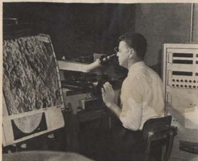
An ACIC cartographer scans moon photographs through a comparator, measuring the length of shadows cast by lunar surfaces. The information he logs, using digitizer at his right and a card punch output writer, is later processed by computers in compilation of USAF Lunar Chart series.
