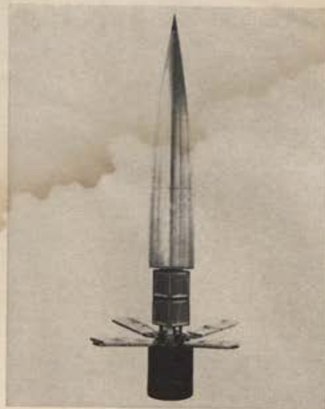
Specially designed Aerobee rocket nose, nicknamed the Venus Flytrap, will be used to collect micrometeorites and noctilucent cloud particles over Canada in upcoming international scientific experiment.
