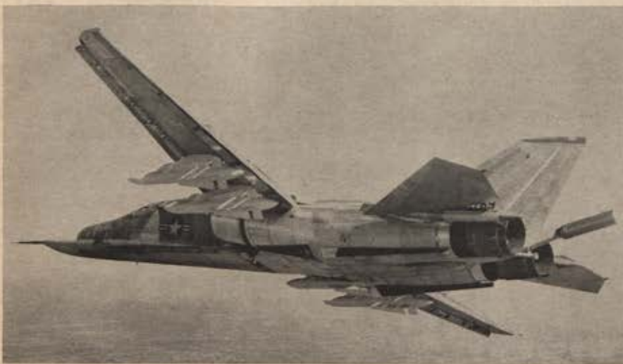
Rotating pylons mounted under the wings of this General Dynamics F-111A undergoing flight tests at Edwards AFB, Calif., swivel to keep the fighter's externally carried weapons parallel to the fuselage during changes in angle of the variable-sweep wing. Canister mounted on tail carries anti-spin chute for test use.
