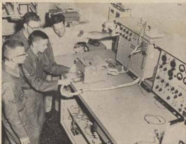
This year the conversion to the F-4C has been mounting at a rapid pace. Here, ATC instructor supervises as students bench-check components of an F-4C control amplifier.
