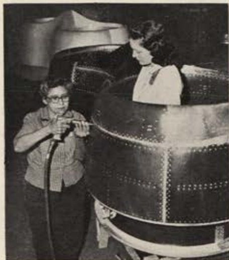
Doris Watkins, a civilian employee of AFLC, seems right at home inside a B-52 engine cowl at San Antonio AMA, Kelly AFB, Tex. She's securing a rivet that's being driven in by Mrs. Stella Derouchie.
