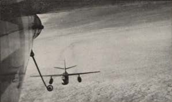
RB-66 Destroyer approaches tail drogue of a KB-50 tanker before hooking up and taking on 5,000 pounds of fuel. Such a refueling normally takes less than 7 minutes.
