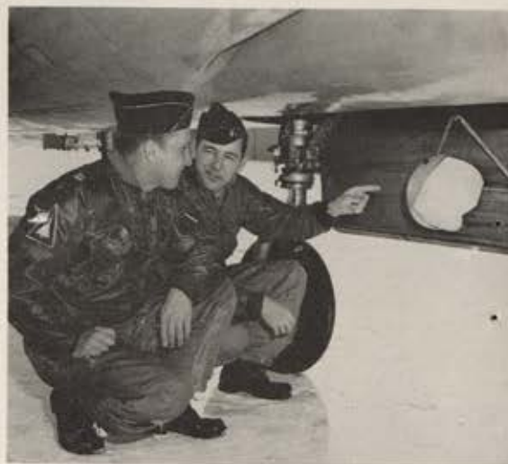
Jet fighter pilots, Capt. Jack Lee, left, and Cleyburn McCauley, discuss side reflector that ground radar "sees" when the F-102 lands using new automatic landing system. The three-sided metal reflector is mounted on the nose wheel well cover of the plane.
