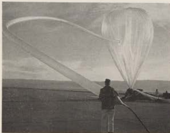
Two-million-cubic-foot plastic balloon is inflated at Holloman AFB, N. M., before being released to carry instrument payload to 102,000 feet in six-hour flight to study cosmic rays above earth's atmospheric screen.
