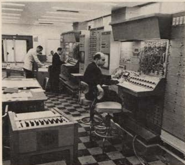
At OAR's Cambridge Research Lab, computer research comprises a large segment of the research program. Shown is a specialized computer designed to trace the pathways taken by electromagnetic energy as this energy propagates from a transmitter to receivers located around the earth.
