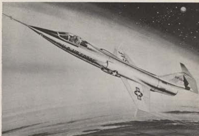
Artist's conception shows a pilot nearing 120,000 feet in rocket/turbojet-powered Lockheed NF-104A during a zoom climb down the high-speed corridor at Edwards AFB. He has begun to use the X-15-type reaction control system, which exhausts propellant from wingtips and nose.
