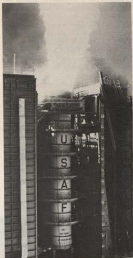
Rocket motor generating one million pound thrust is successfully tested in inverted position at Coyote, Calif., July 20. Two of these motors, built by United Technology Center, will make up the first stage of the Titan III-C space booster, scheduled to launch USAF's Dyna-Soar into orbit in 1966.
