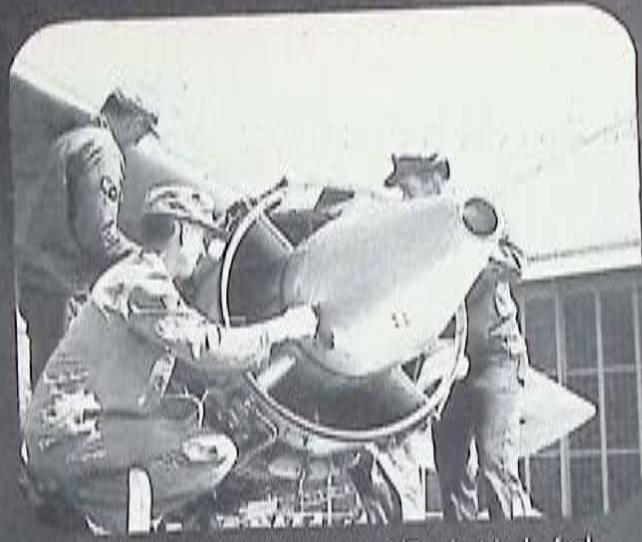
0906 Quick-disconnects of J47 electrical, fuel, and oil lines are completed.
