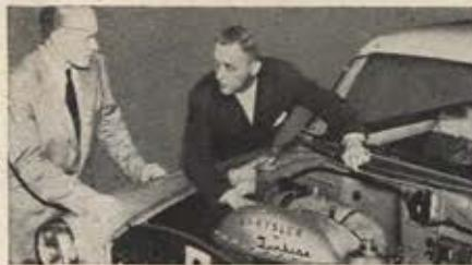
Simplicity has been achieved in the Chrysler gas turbine engine. It is 200 lbs. lighter, has one-fifth as many moving parts as the piston engine it replaces. It is air cooled, eliminating all radiator and liquid cooling components.
