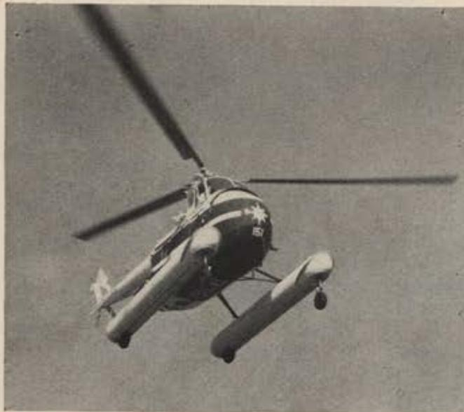
**JAPAN**—One of eleven Sikorsky S-55 helicopters built for Japan is pictured above being test flown with new flotation gear. This model is for Japan's official Maritime Safety Agency. Other Sikorsky S-55s are being delivered for service with air and ground branches of that country's National Safety Agency and Maritime Safety Agency.
