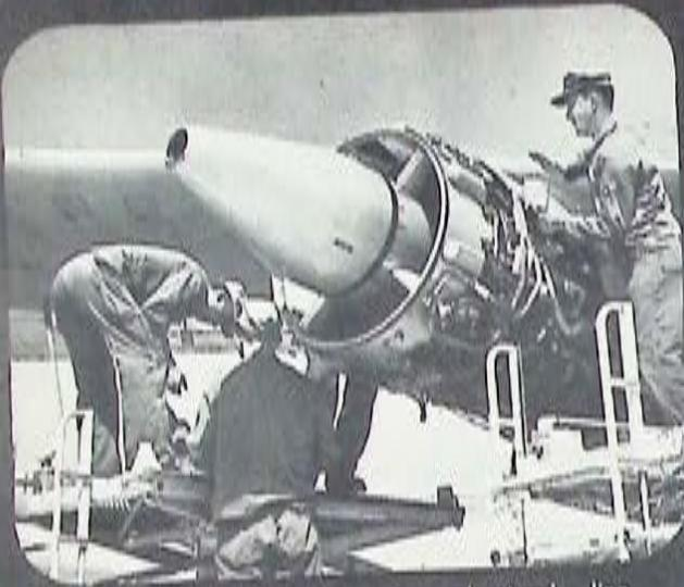
0900 Stepping up on their work stands, line crew removes outboard engine cowling.
