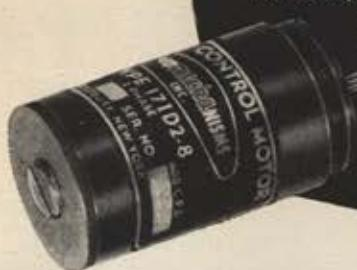
Servomechanisms, Inc. Type 171D, for use with the amplifier, is a damped-control motor whose control winding is the output load for the amplifier.
