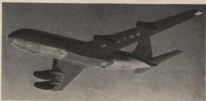
Boeing's new all-jet Stratotanker-Stratoliner, now undergoing extensive flight tests. Statistics: span—130'; length—128'; gross weight—190,000 lbs.
