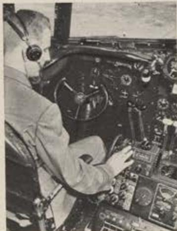
**1946** United Air Lines installed Sperry A-12 Gyropilot on four-engine fleet to insure precise automatic instrument approaches to airport runway. UAL President, W. A. Patterson, considered installation . . . "a definite start in eliminating weather as an obstacle to airline operations."
