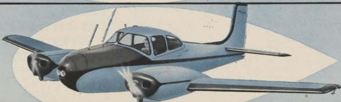
Riley Twin Navion Conversion. 4-place executive plane powered by two 150-h.p. air-cooled Lycoming engines.
