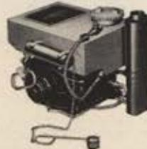
Prime movers interchangeable—mittens on—in just ten seconds! Engine preheater "cigar lighter" torch gets engine going within 3 minutes at -65°F. Alternate power source is 115/230 volt, AC 60 cycle single phase motor.
