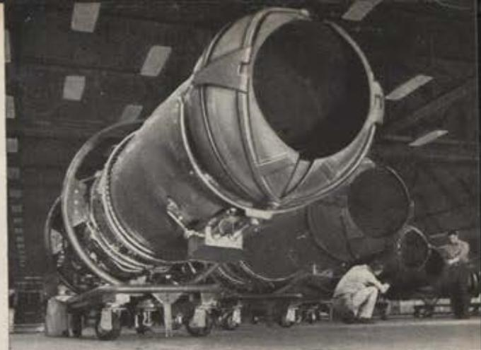
AUTOMATIC CONTROL of the variable area nozzle (illustrated above) regulates exhaust velocity and temperature.
