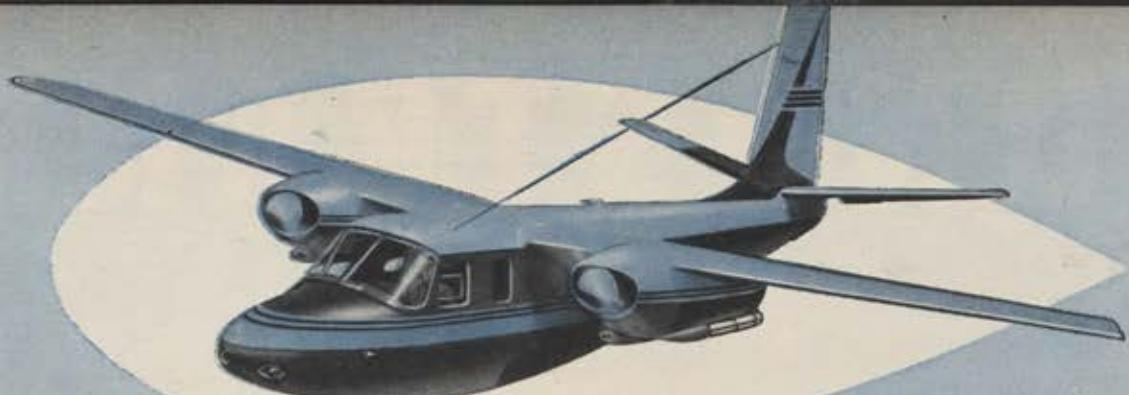
Aero-Commander. Seats 6. Powered by two 260-h.p. Lycoming air-cooled, geared engines.
