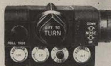
MODEL L-2: Controller for Autopilot System for aircraft in the professional, executive and light plane class.
