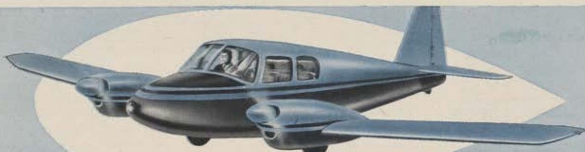
Piper Apache. Seats 4. Dependably powered by two 150-h.p. air-cooled Lycoming engines.
