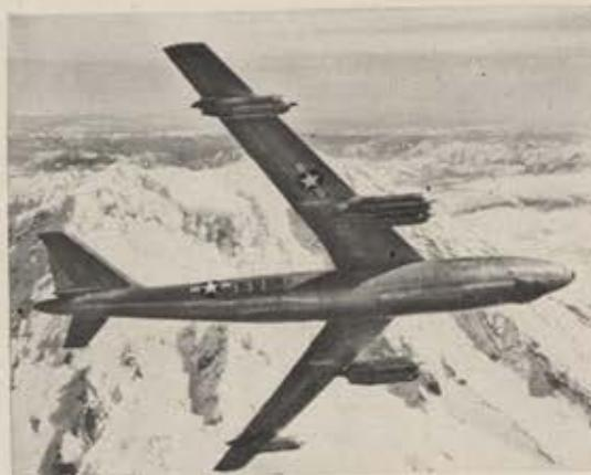
**1953** USAF's Boeing B-47B is equipped with Sperry Gyropilot, combining the latest in gyroscopic, servo, and signal system techniques. This automatic flight control system meets strategic requirements for high-altitude, long-range missions and automatic precision bombing runs.
