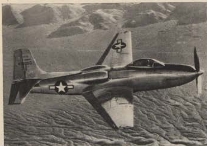
Convair XP-81, first turboprop-powered aircraft to fly in U.S., powered by TG-100, first American turboprop.
