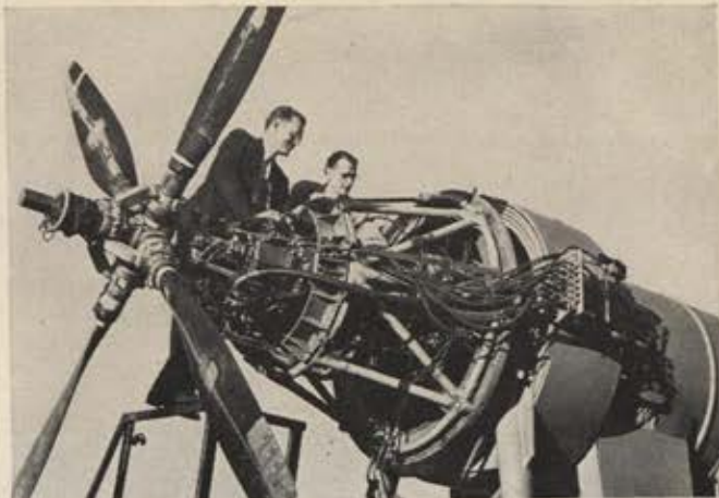
Design engineers Alan Howard and C. J. Walker, inspect an early TG-100 turboprop on test stand in Schenectady.
