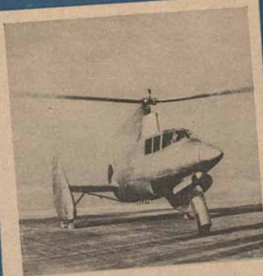
Latest in helicopters , the French SE-700. Note retractable nose gear, fins housing rear main wheels.
