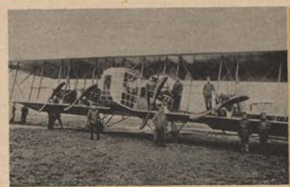
The 102-foot Ilya Mourometz completed in 1914 had 220-hp Renaults. (Below) Germany's 115-foot DFW bomber, completed in 1918. Eight 270-hp engines drove four propellers.
