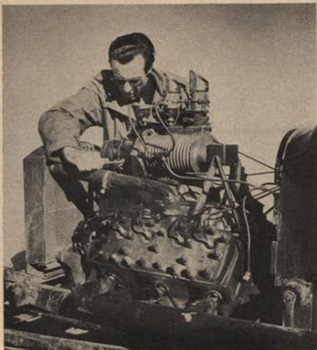
Hot-rock engineering. Don Blair of Southern Pasadena adjusts the interlocking-vane type supercharger, which added sufficient compression to jump his Ford V-8 powered racer to a speed of 134 mph.
