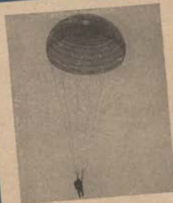
AAF ribbon parachute, designed at Wright Field for high speed.
