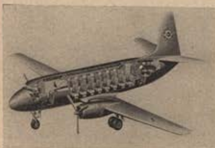
Cutaway of Northwest's Martin 303 shows pressurized cabin for 38 passengers, lounge.
