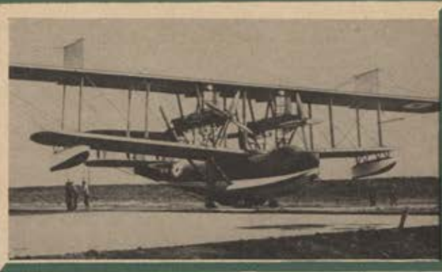
Fairey's Titania, built in 1923, spanned 136 feet. Powered by four 600-hp. Rolls-Royce Condor engines and designed to succeed the veteran Cromarty boats, this patrol bomber was built for long-range deep-water operations. Loaded, it weighed over 31,000 pounds.
