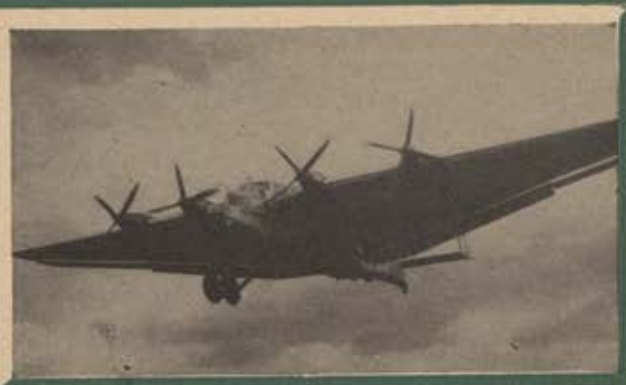
While only a few G-38 Junkers transports were built by Germany, the ship proved among the first financially successful gargantuas of the early '30s. Powered by four 800-hp Diesel engines, it weighed nearly 60,000 pounds and cruised at better than 125 miles per hour.
