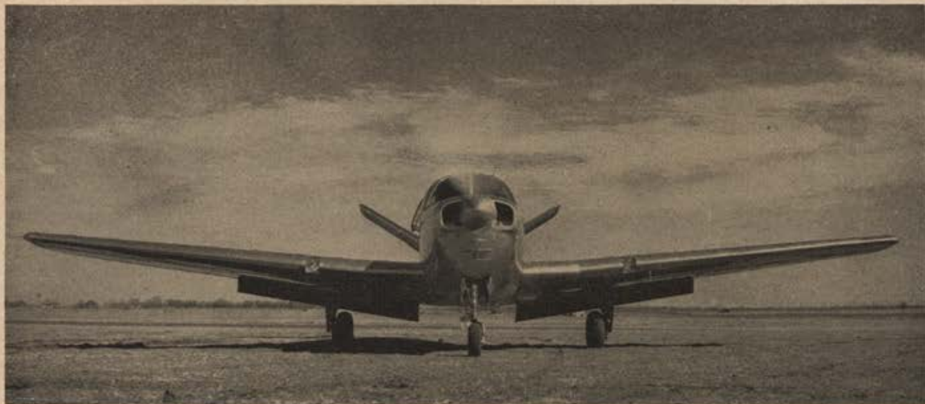
With full flaps Beechcraft Bonanza lands in less than 300 feet. Wide tricycle tread, castoring nose wheel aid soft field landings.
