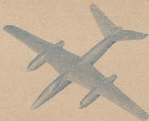
This proposed attack-type carries two prop-jet engines under the wing, and a turbo-jet in the tail for combat-emergency power. Right,
