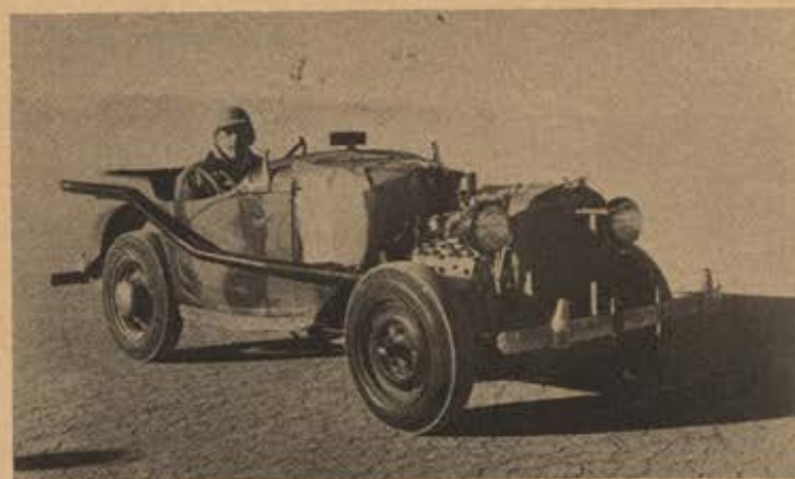
Veteran Jack Rutledge races his composite Ford 60, with a 1937 block. Note the old-vintage Austin parts, used in rear of body.
