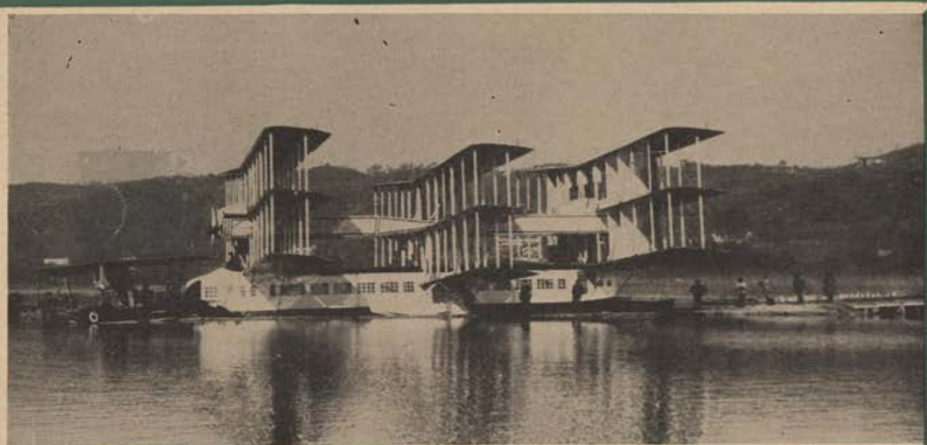
Coproni built the triple-triplane in 1921. It was supposed to carry 100 persons 5,000 miles. The boat was 70 feet long and power was provided by eight 420-hp U.S.-built Liberty engines. This giant cracked up on its first landing after a flight to an altitude of 200 feet. The conventional tail was totally absent from the design. Rear wing hinged surfaces on the back set of airfoils acted as elevators. Flat vertical surfaces between the rear triplane's members acted as rudders. Triplanes declined after this failure, chiefly for structural reasons.
