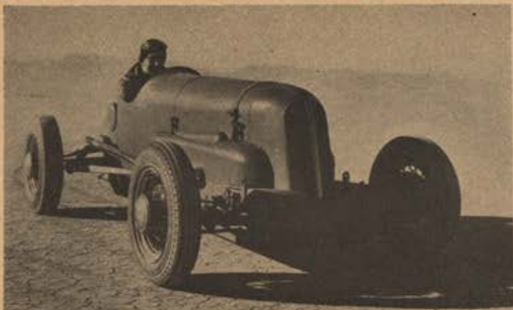
This fine specimen, owned by former Merchant Mariner H. L. Markham, is a 1928 model chassis housing a 1933 Ford block.
