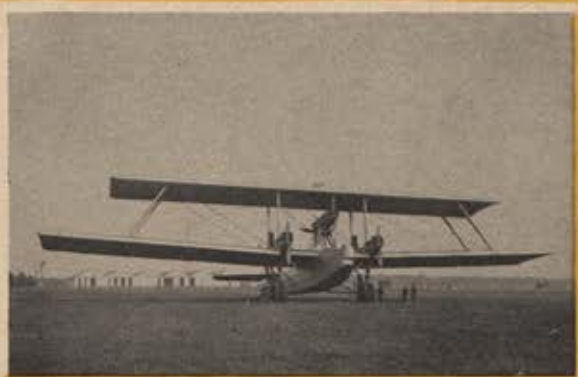
Caproni's Ca 90B was Italy's entry for the world's biggest in 1929. Span 159 feet. It had six 1,000-hp Fiat engines.
