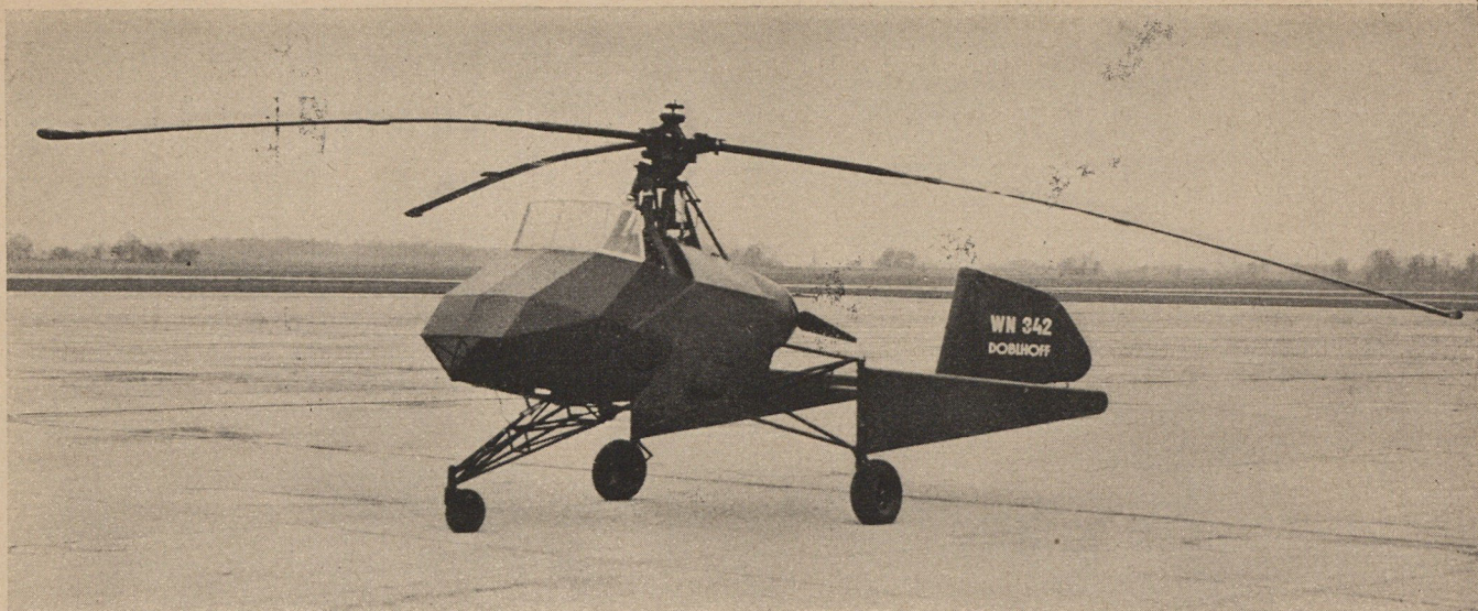
One of the most unique aircraft was the jet-propelled helicopter, WN 342 which employed jet rotors for ascent and descent.
