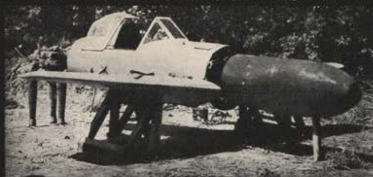
Fairing removed, showing mount and warhead which contains trinitroanisole.
