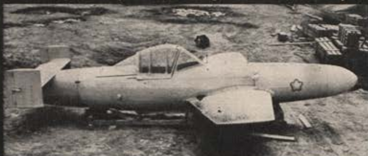
Baka is made of aluminum and plywood, has armor plate around cockpit.
