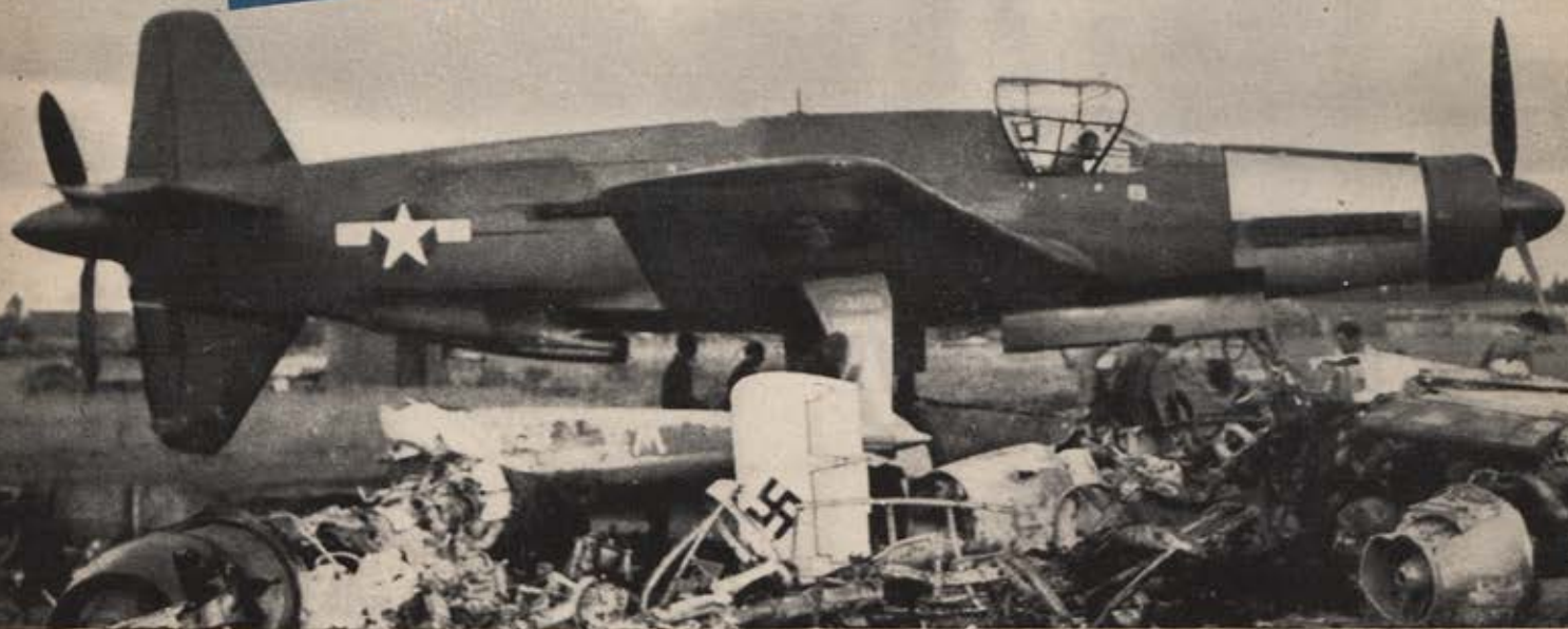
This Dornier 335, shown with American markings, is driven by a propeller mounted in the front and by another installed in rear.
