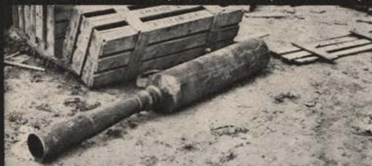
Baka rocket tube contains six grains of propellant charge in its motor.
