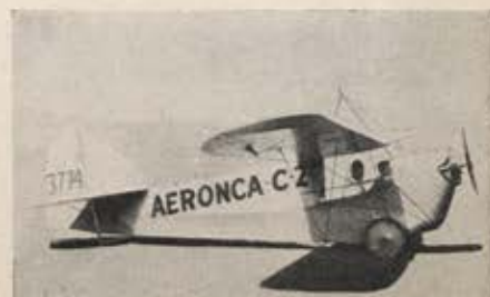
Styled as "America's First Light Airplane," this Aeronca was powered with 28 hp engine.
