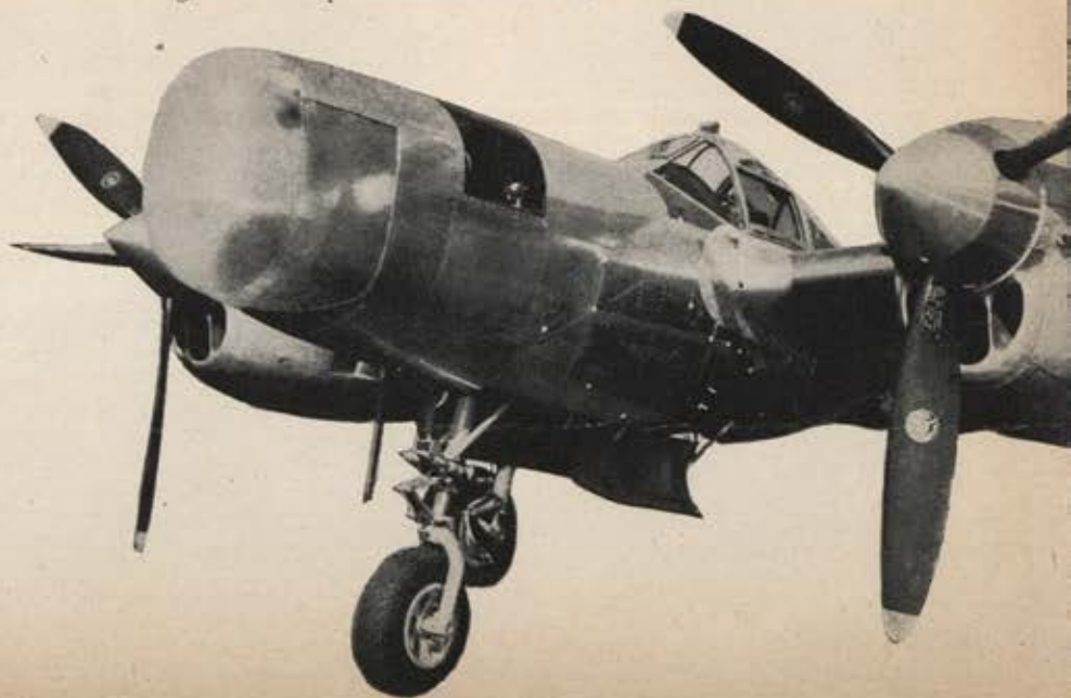
P-38 with special equipment in elongated nose is pathfinder for formation.
