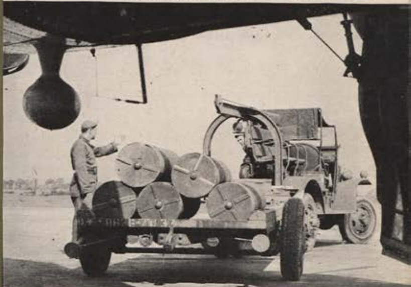
▲ Ready to be hoisted into B-17 are five 300-pound leaflet bombs. ▼ Leaflets are scattered to winds when bombs split open in air.
