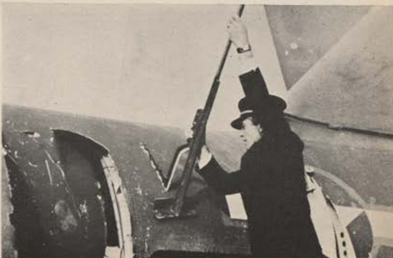
Operated like an outsize can opener, this tool slices through the fuselage of an airplane to free crewmen. Shearing action reduces sparks.
