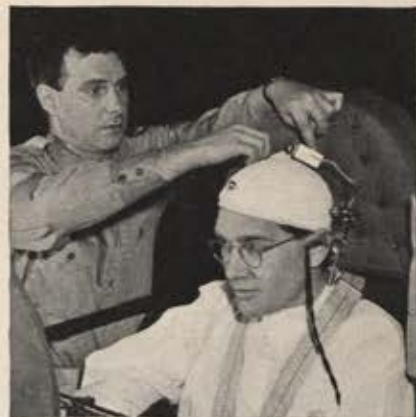
Final adjustments are made on brain wave recorder cap before subject is given experimental spin in centrifuge at Wright Field.
