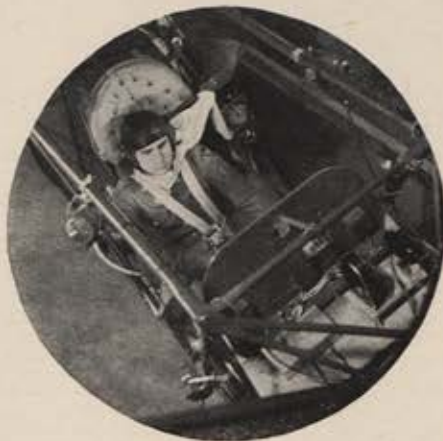
During actual tests in centrifuge, cab swings outward or inward so subject's body is parallel to floor. Cab is tilted only partially in this photo. Movie camera on frame records subject's facial changes.
