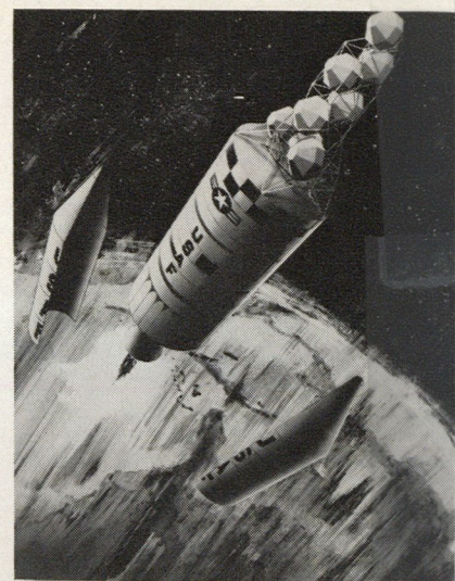
Artist's sketch shows shroud as it falls away to expose eight satellites borne aloft by Titan IIIC booster. In near-stationary orbit, satellites were released one by one to form a necklace around earth.
