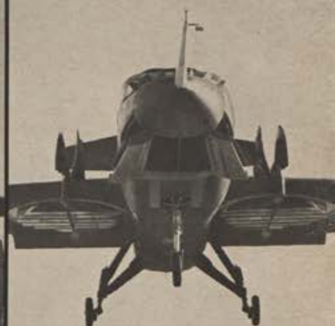
GE-Ryan XV-5A lift fan system J85 engine
