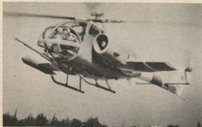
US Army's XH-51A compound helicopter, which recently set world speed mark for rotorcraft of 272 mph, made its debut at Paris show. The Lockheed rigid-rotor aircraft is thirty-two feet long, with a rotor thirty-five feet in diameter.
