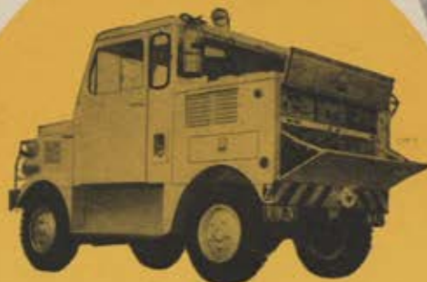
Self-propelled, multi-purpose, ground-sup- port unit . . . for starting, servicing, test- ing and towing. Provides A.C., D.C., hydraulic and pneumatic power.
