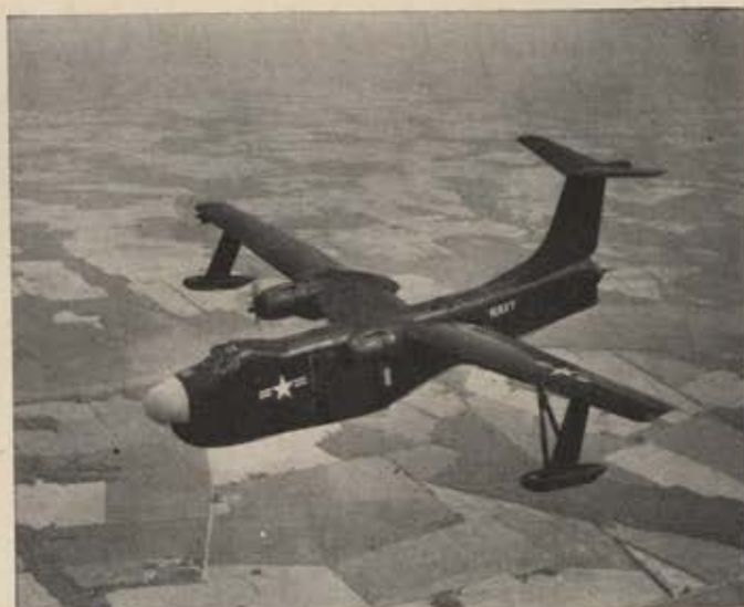
▲ Speedboat bow and high "T" tail better suit the new version of the Martin Marlin for anti-submarine work.
