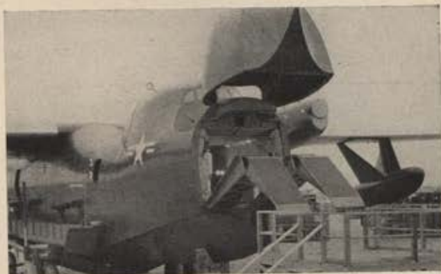
▲ The ramp on Convair's R3Y-2 unfolds, showing how the "Flying LST" will land men and guns on assault beaches.
