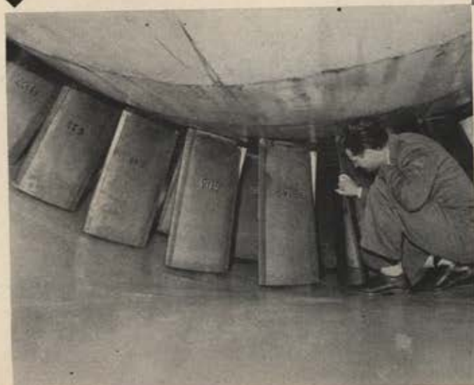
▲ A Boeing engineer checks the laminated glass fan blades now being used in the company's transonic wind tunnel.
