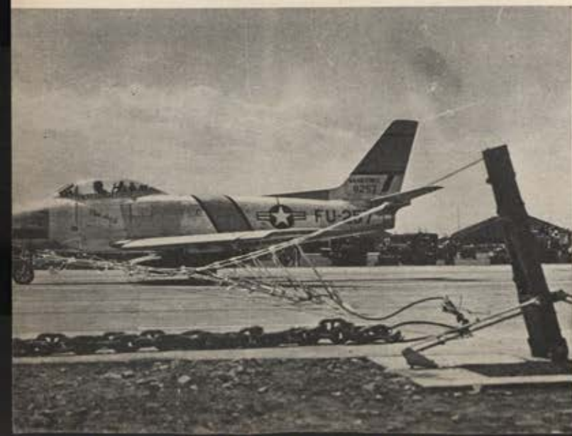
Camera catches F-86 (top) as it contacts runway net, while (below) it trips the arresting cable which engages the main landing gear. Dragged along ground, the chains in foreground finally stop plane.
