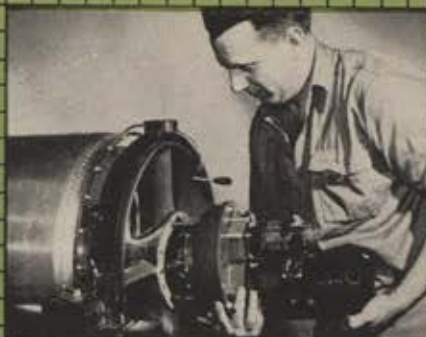
ACCESSORY SECTION containing essential controls, is quickly removed and replaced without special tools.
