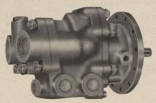
Pesco Model 011799 Unloading Gear Pump. Weight 8.6 lbs. Maximum continuous operating pressure 1500 p.s.i. Capacity 2 g.p.m. at 1500 r.p.m. Features Pesco's exclusive, patented "Pressure Loading" principle. Other models available for pressures to 3000 p.s.i.
