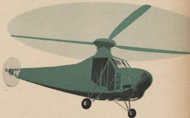
Aeronautical Product's A-1 mounts engine forward instead of under main rotor as in other such craft.
