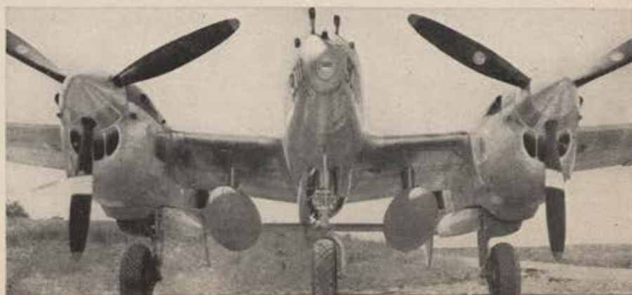
This P-38 is all set to drop 330-gallons of flaming jelly which is almost non-extinguishable.
