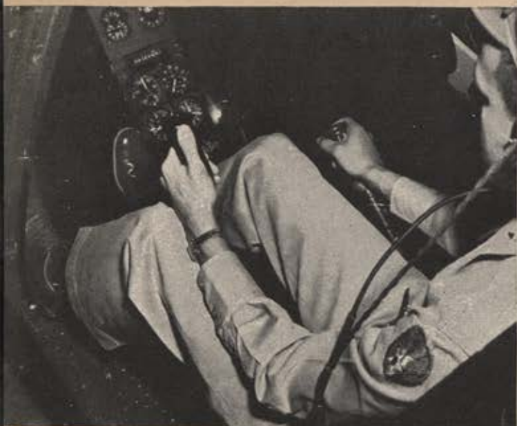
Controls of the R-6 Helicopter. In the pilot's left hand is the joy stick; right hand, pitch stick with throttle handle.
