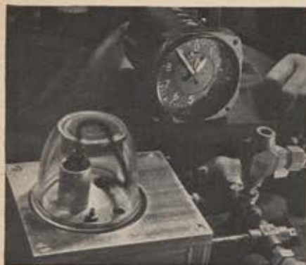
Smallest pressure chamber yet devised is used by AAF to simulate wide range of altitudes, temperatures in testing radio parts.
