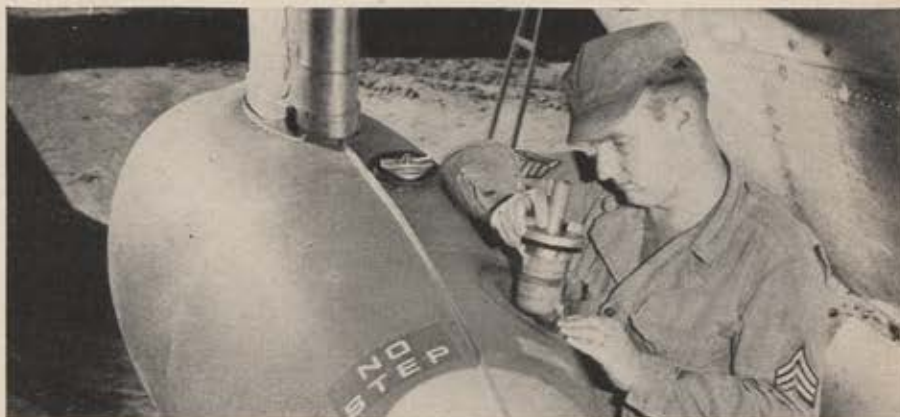
Detonator fits into gas cap hole, has small fuze that explodes upon impact, firing jelly.
