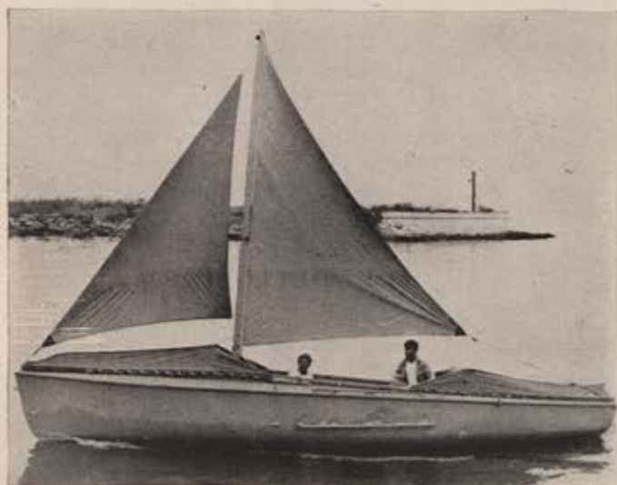
To save gasoline, the boat can be converted into a sailing sloop by use of its portable, 20-foot mast and 145 square feet of mainsail and jib. Stowed food and equipment are ample for a 1500-mile voyage.
