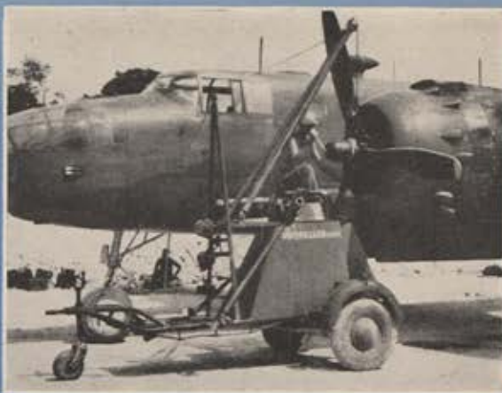
Tech. Sgt. Clarence Lavender put a boom and hoist on a standard dolly; now mechanics are able to drive out to a plane, install or remove the prop in one operation.
