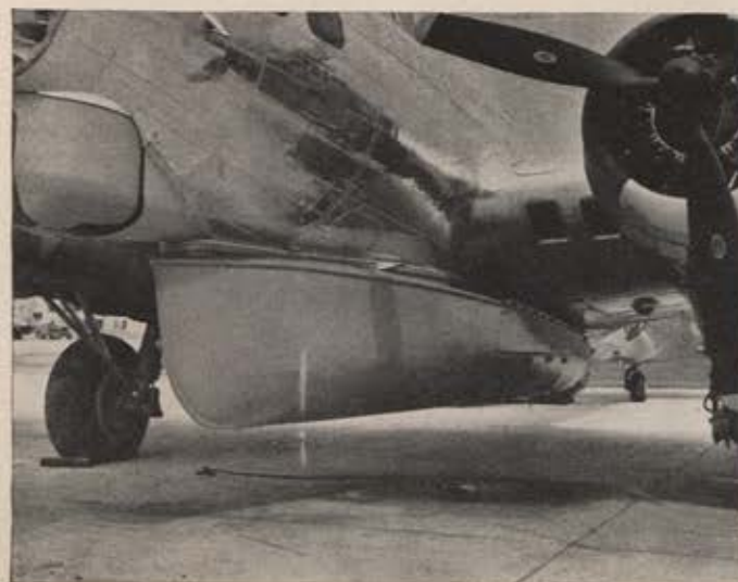
In carrying position, the Flying Dutchman hugs the fuselage of the plane. The fit is so snug and the boat's lines, with prow forward, are so smooth that the burden reduces a B-17's speed only eight mph.
