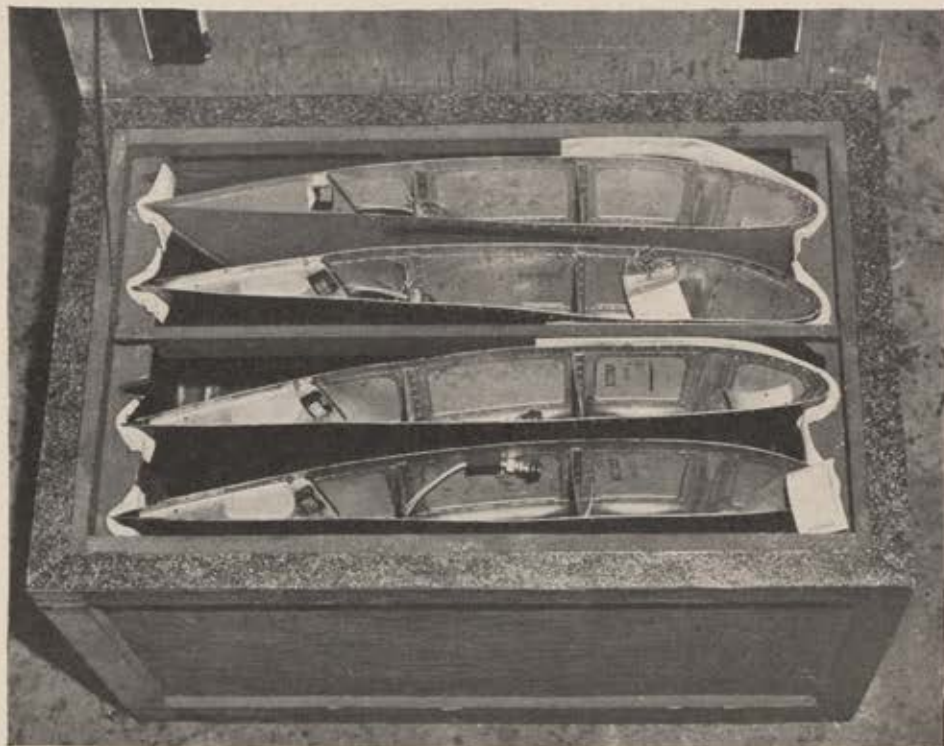
To replace damaged wing-tips, boxes of new ones are sent to advanced bases in compaks. Removal of one wing-tip does not disturb the others, for each is anchored and cushioned.
