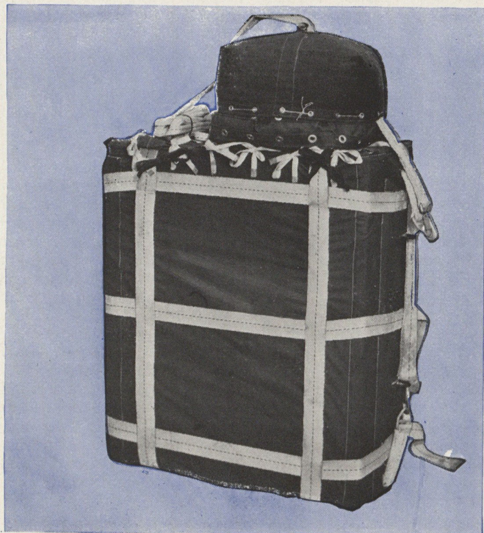
The A-4 delivery container consists of two general purpose cases with cargo parachute on top.
