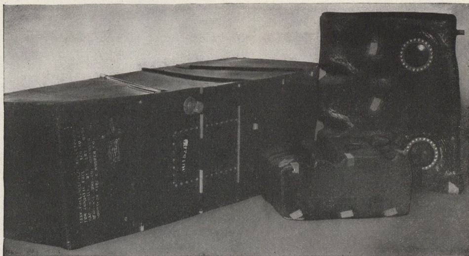
Above are some typical fuel cells. Note that all fittings are covered with masking tape. Inspection doors are safety wired and cells are properly stenciled for identification.
