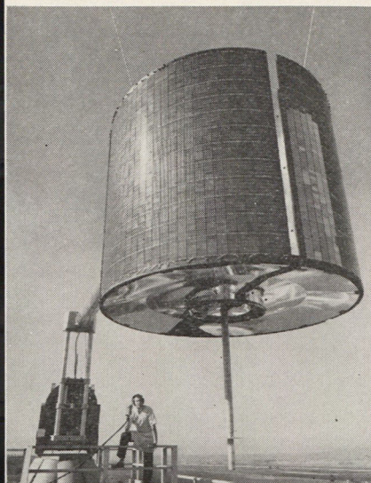
Early Bird, at left, built by Hughes and deployed for COMSAT Corporation over the Atlantic, is an advanced version of the Syncom system and is providing telephone and television service between Europe and America. A Pacific Early Bird will soon provide a similar service in that area.
