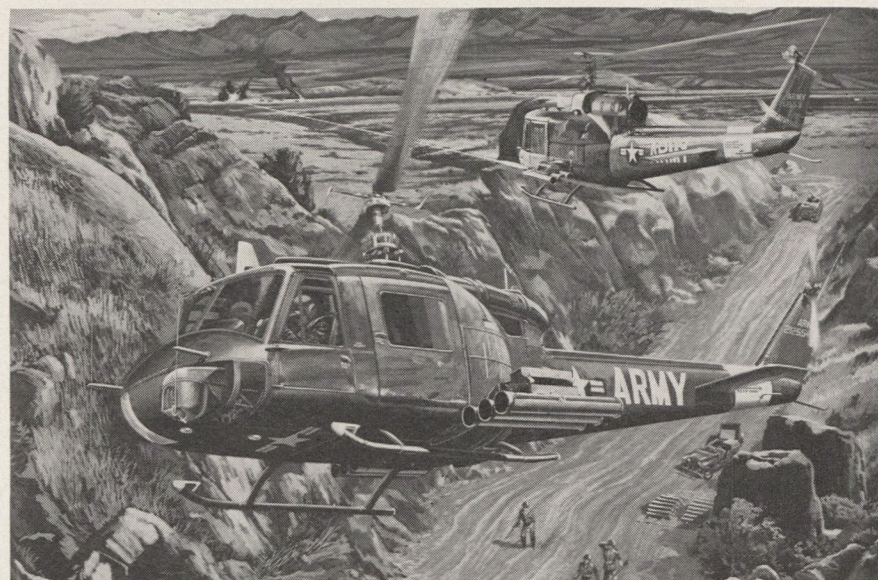
Artist's sketch shows U.S. Army UH-1B Huey helicopters equipped with TOW anti-tank missiles. Gyro-stabilized sight being developed by Hughes Aircraft Company, which also manufactures TOW missile, will enable gunner to keep weapon aimed on enemy tank, armored vehicle, or ground emplacement despite helicopter's evasive actions.
