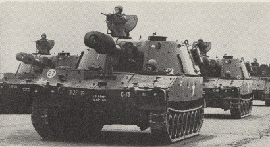
U.S. Army's M-109 self-propelled tracked vehicle, carrying a 155-mm howitzer, will be coproduced in The Netherlands under a recently-signed agreement with the U.S. About 100 M-109s will be purchased at cost of $14,000,000. The 155-mm howitzer swings in full circle with elevation from minus 3° to plus 75°.
