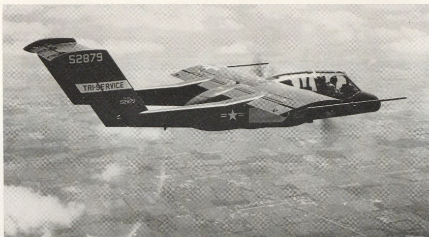
FACs in Vietnam are eagerly awaiting the arrival of the North American OV-10A in mid-1967 to replace the Cessna O-1s now in use. The twin-engine reliability and very fine rate of climb of the OV-10A, which rivals that of the World War II P-51 Mustang, are high on the list of priorities for FAC pilots in combating Viet Cong antiaircraft fire.
