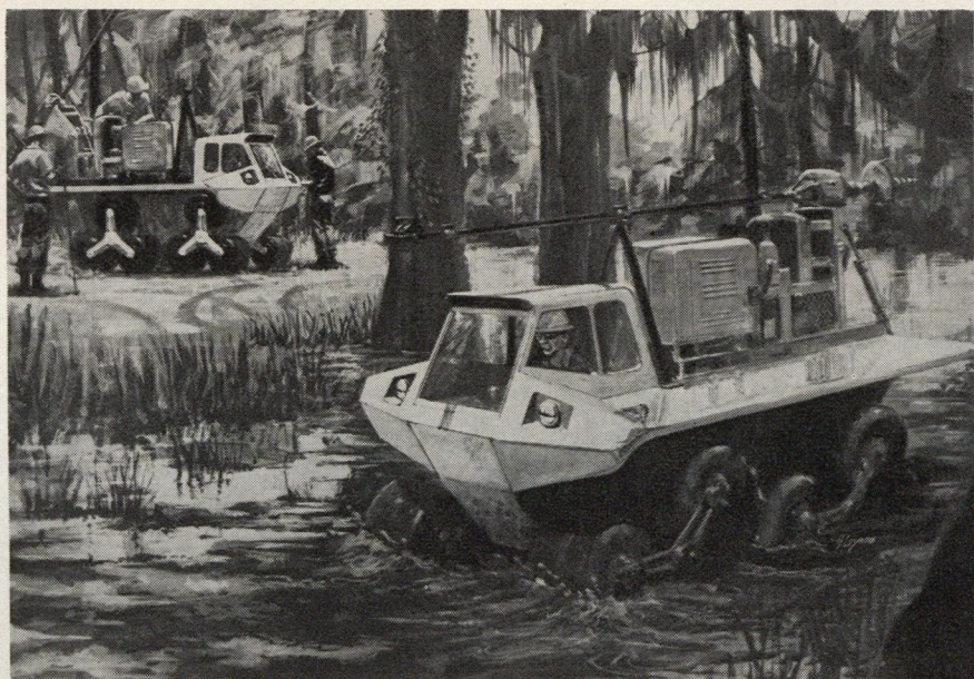
Wheels within wheels propel this Lockheed TerraStar vehicle over paved surfaces, mud, and swamps, or through water. Each of 4 major wheels is made up of 3 minor wheels mounted radially on spokes around main axle. On hard surface, vehicle runs on pairs of minor wheels. In mud or water, TerraStar "paddles" along by revolving major wheels.
