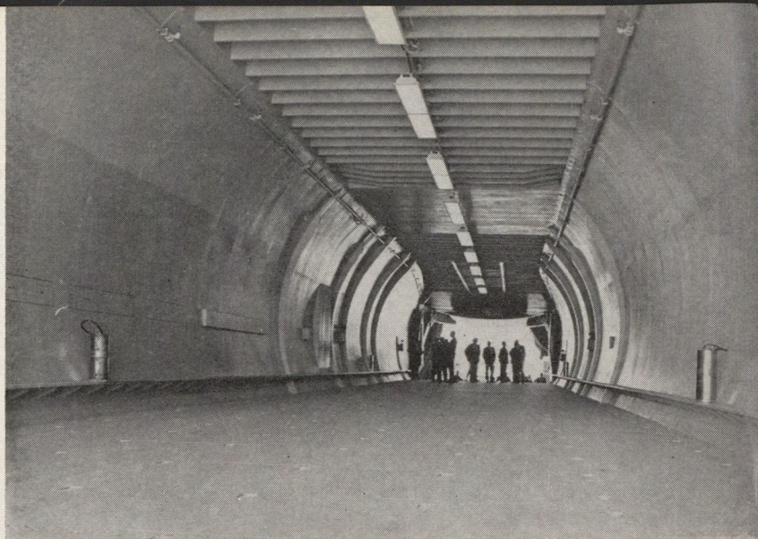
The mockup of the 121-foot-long (36.9 m) C-5A cargo compartment looks like a huge tunnel in this photo, taken from the rear ramp. The compartment is longer than the Wright brothers' first flight at Kitty Hawk. A proposed commercial version of the C-5A, called the L-500 by Lockheed, would have 3 decks and carry some 900 passengers. Military version will carry 75 troops on top deck, in addition to cargo load.
