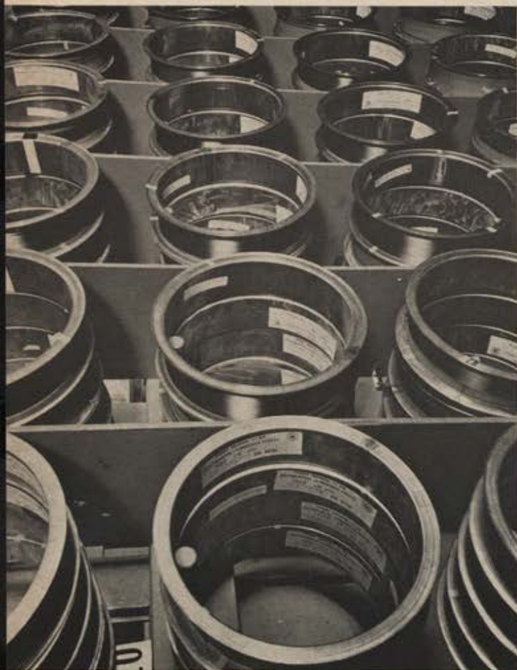
Miles of boron filaments are shown here at the Richmond, Va., pilot plant of Texaco Experiment Incorporated. Originally developed for the Air Force as a component for high-energy fuels, boron now is considered one of the most promising advanced materials for aeronautics. These reels are being shipped to other contractors for evaluation.
