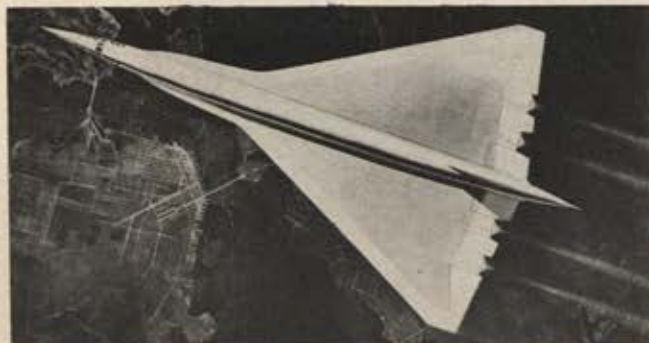
Lockheed's design for the SST relies on a double-delta, fixed-wing configuration to cope with aerodynamic requirements of supersonic flight, transonic transition, and take-off and landing. Careful contouring of wings is said to lower sonic boom potential while increasing lift-drag ratio.
