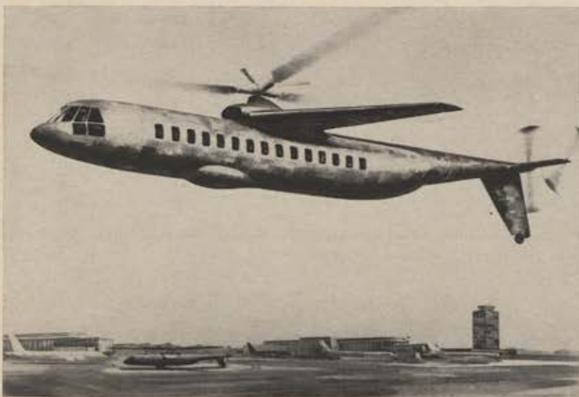
This artist's conception shows Lockheed's sixty-passenger "Metroplane," which could be flying within the next five years. A winged rotorcraft, this vehicle is said to be capable of speeds up to 375 miles per hour. Following vertical takeoff, the aircraft would fold its rotorblades back for conventional winged flight. "Metroplane" would be more economical than present shuttle service.
