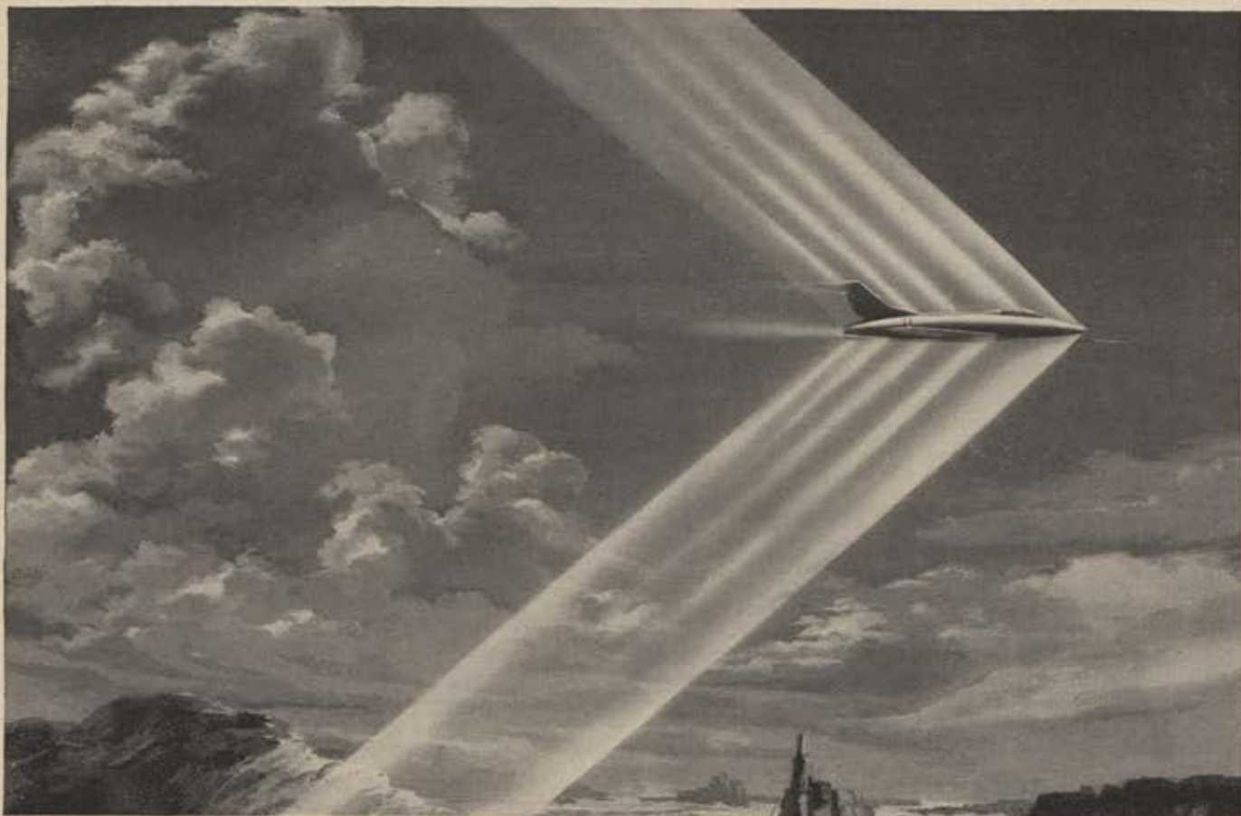
A new F-100 Super Sabre in level flight smashes through the sound barrier over a remote test area creating a gigantic shock wave—the Sonic Boom.
