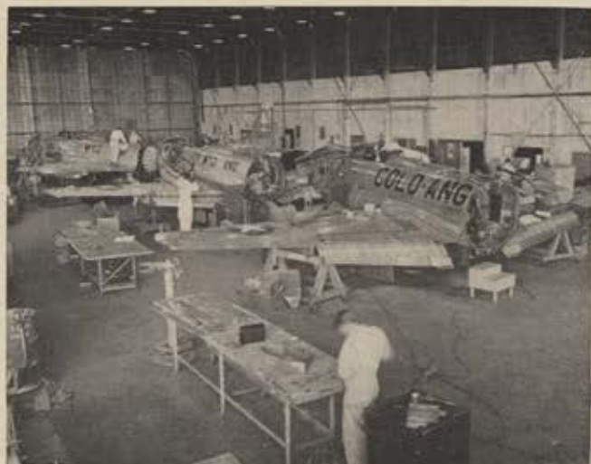
Some 180 Lockheed F-80 jet fighters assigned to the ANG are being modified at the plant. Above, work in progress.
