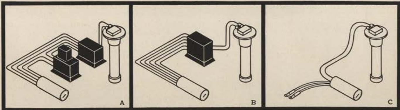
**Fuel gaging progress:** Early gaging system (A) had four units. The 1952 system (B) incorporated bridge and amplifier into a single unit, reduced weight almost 15%. Avien's Two-Unit Fuel Gage, now being introduced (C) repackages the system with further miniaturization of components, this time reducing weight by 50%.
