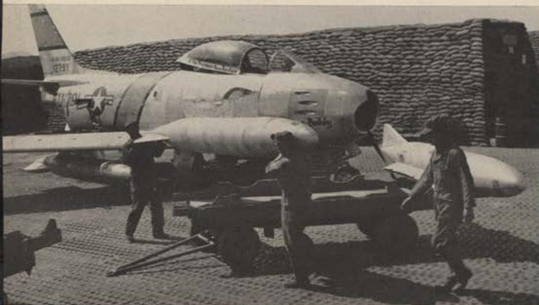
No short rations for an F-86! Ground crewmen see that the Sabre, parked in its sandbag revetment at a forward base, has plenty of fuel for the trip to MIG Alley and back. Tanks are jettisoned when Sabre meets MIG.
