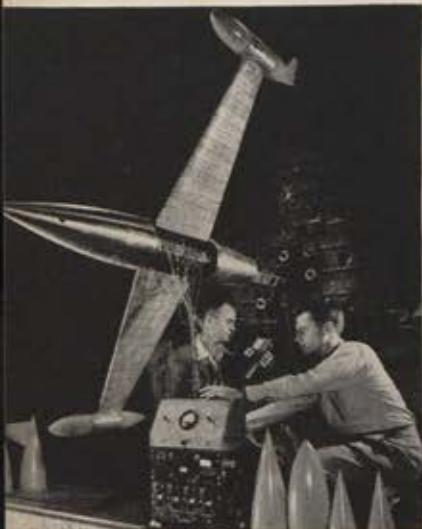
NACA's shops turn out accurately scaled, highly instrumented models to gather aerodynamic information on plane and missile configurations. At left, a dynamic flutter model is instrumented. Plastic cones of varying shapes (right) are for high-speed airflow studies.
