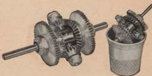
Precision miniature differentials are designed for applications where space is at a premium without a sacrifice in accuracy. Low breakaway torque, adjustment for wear and dual planetary gears for high torque capacity are combined in this design to give maximum performance in a minimum of space.
