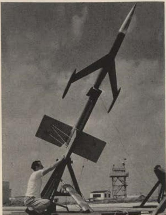
Above, one of a series of models flown at Wallops Island, Va., to determine best shape, size, and location for fuel tanks on a swept-wing fighter. Left, a similar model, spun from magnesium sheet less than a tenth of an inch thick, is assembled. Right, nose section for a supersonic model is hot-spun from magnesium on a lathe.
