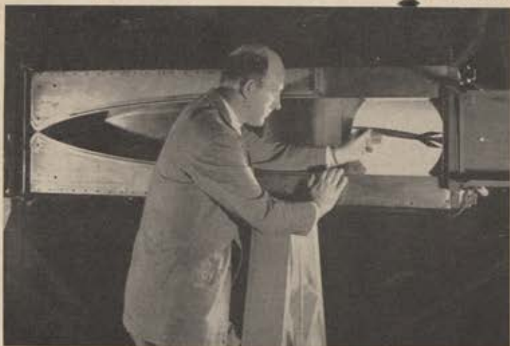
At the other end of the scale is this tiny 11-inch hypersonic tunnel to study the nature of airflow at from five to ten times the speed of sound. Photo shows side plate removed, exposing nozzle at left, a narrow slit through which air enters under great pressure. The air then expands rapidly and rushes past the model.
