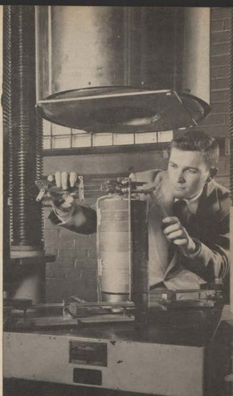
Titanium, which will replace aluminum alloy in many parts of highspeed aircraft, is tested for strength at high temperatures (above). The full-scale tunnel (below) was originally built to test full-scale airplanes at flying speed, now tests high-speed planes at landing speeds. Entrance cone measures 30 by 60 feet.
