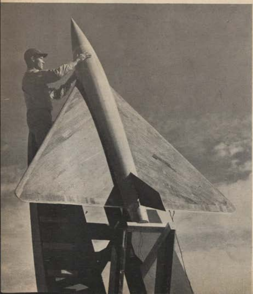
A radio telemeter (above) is installed in a research model to be flown at the Wallops Island research station. Using several channels, it transmits aerodynamic information to a ground station. Delta-wing model (below) is prepared for launching to obtain aerodynamic data on high-speed flight design factors.
