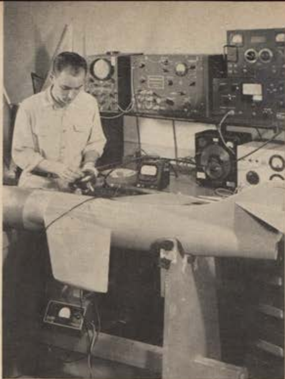
Circuits of the miniature instruments installed in a rocket propelled research model are checked at the Instrument Research Division at Langley Lab.
