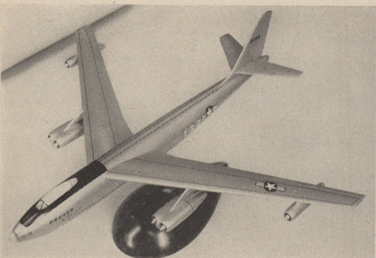
Above, the final model—the one actually used in wind tunnel tests before building a prototype. Above right, five years later a contract has been let and production at Boeing begun, but 47 still can't be counted as part of air strength in being.
