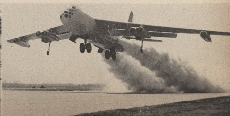
Below left, the first completed B-47A Stratojet rolls off the assembly line for delivery to the Air Force. This was March, 1950—six and a half years after initial study had begun. Below, the Stratojet takes to the air with JATO.
