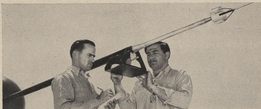
Needle-like boom (above) is installed in nose of Northrop XF-89 to pick up dope on speed, altitude and yawing action in the calm of the air ahead of the plane. And now it's track-tread landing gear for the massive B-50 Superfort. The picture below was taken during the 164,000 pound plane's first taxi runs.
