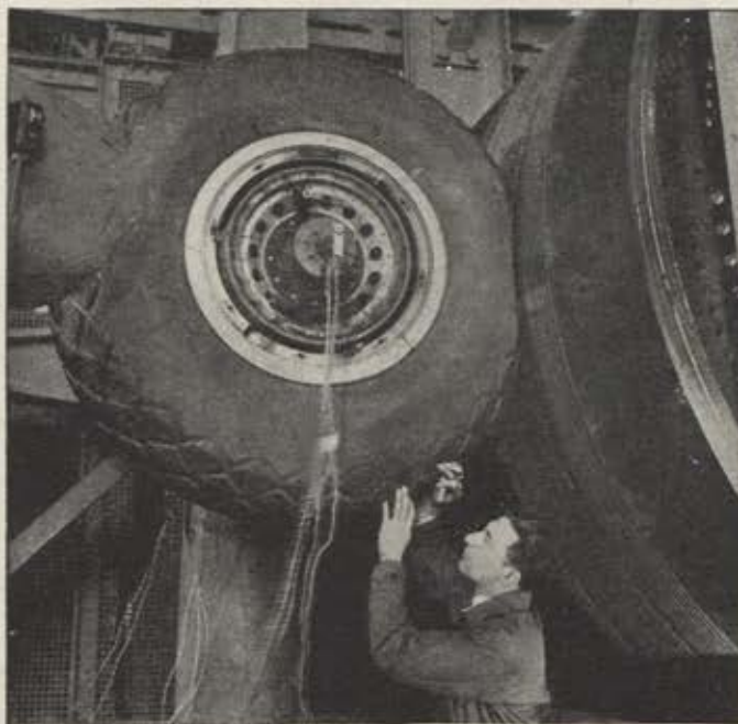
Inertia wheel tests such as this provide necessary information for improvement of aircraft brakes and tires. Below, a workman, using a hypodermic needle, checks the heat generated between tire and wheel.
