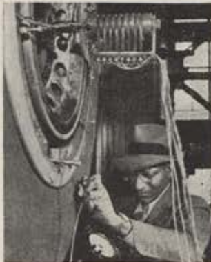
Inertia wheel tests such as this provide necessary information for improvement of aircraft brakes and tires. Below, a workman, using a hypodermic needle, checks the heat generated between tire and wheel.
