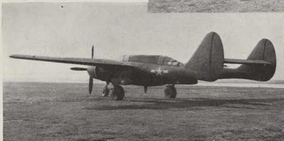
Two views of the Black Widow night fighter reveal its similarity to the Lightning, with several other features distinctive from all other planes in combat. It is larger and has greater firepower than any AAF fighter craft.
