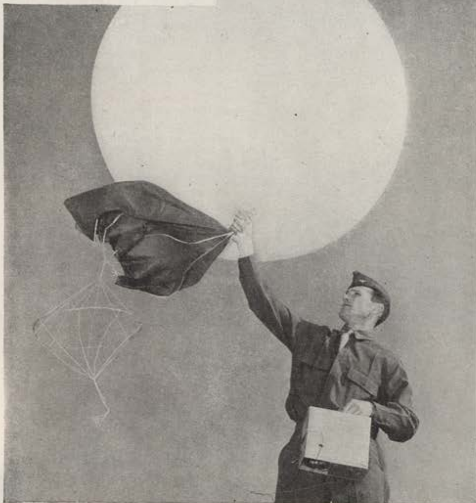
The small package held by this cadet is a radiosonde, a miniature radio broadcasting and weather station which is sent aloft by hydrogen balloon to record and transmit information on temperature, atmospheric pressure and humidity. At 30,000 feet it descends by parachute.
